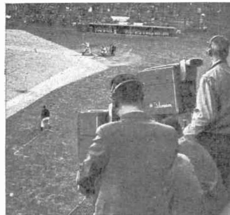
Several television cameras strategically located cover the baseball diamond to bring you a close-up of the action wherever it occurs. The engineer can switch from one camera to the other for the best view. Here are two of the super-sensitive RCA Image Orthicon television cameras used by NBC's New York station WNBT in televising all the home games of the New York Giants this season.
