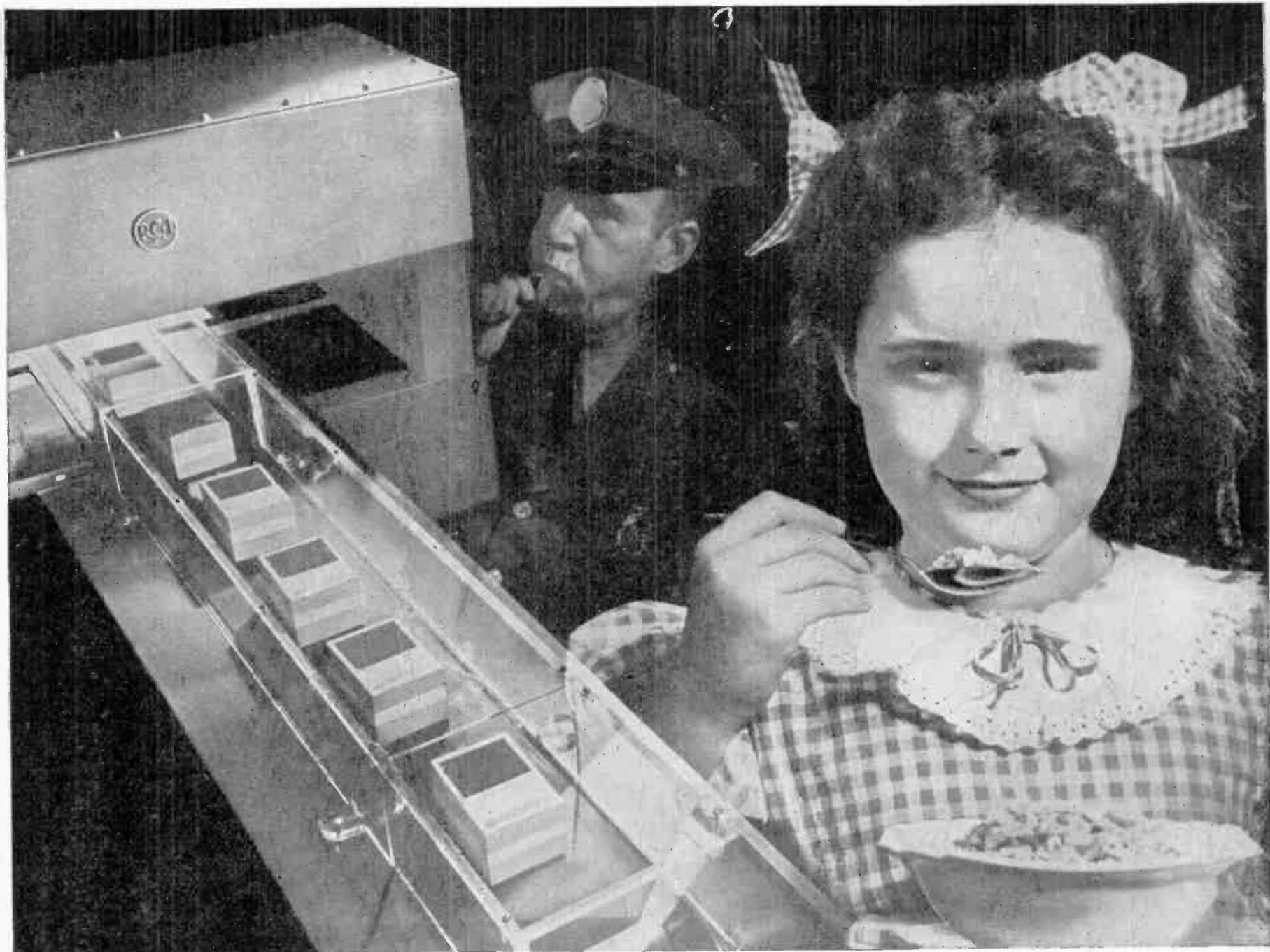
The RCA Metal Detector "blows the whistle" on any particle of metal that may have crept into the package.
