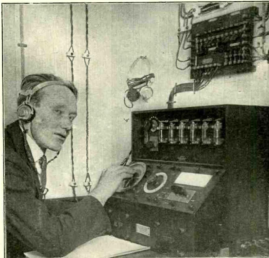
(Above) The latest type of Marconi direction finder—an aerial of two loops at right angles to each other—which determines the direction of messages from shore stations and ascertains the exact location of a ship in a fog. The instrument is one of the new wonders in radio.
