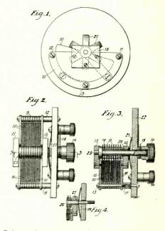
Schematic diagrams of the Johnson electrostatic condenser which, when rotated, may prevent short circuits. The invention provides improved means to protect the movable rotor from accident, against any adjustment.
