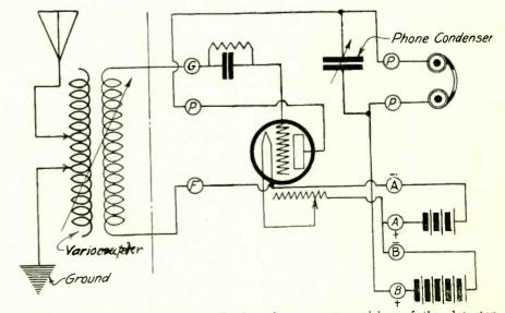
Figure 3-Schematic diagram showing the necessary wiring of the detector and control panel. Suggested by Frederick J. Rumford. Drawn by S. Newman.
