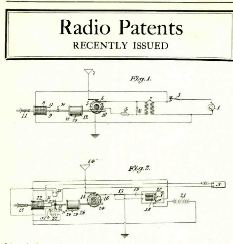
Schematic diagram illustrating the circuits of the invention of John Hays Hammond, Jr., to perfect conversation, without interference, between two stations, regardless of the number of stations on the same wave-length.
