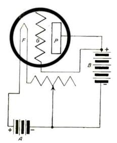
Figure 3—Schematic diagram similar to Figure 2. The difference is that the grin of the tube is connected with the plate circuit. This renders the plate and grid positively charged. This would tend to make a negative filament with grid and make a negative filament with grid and plate positive. Suggested by G. W. May. Drawn by S. Newman.
