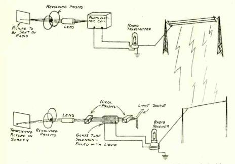
Schematic diagram showing the operation of the invention of C. Francis Jenkins which not only transmits photogaphs by radio but, the inventor claims, will transmit motion-pictures as well. Follow the course of the diagram from the upper left-hand corner to the right. downward, and then left to the lower left-hand corner.
