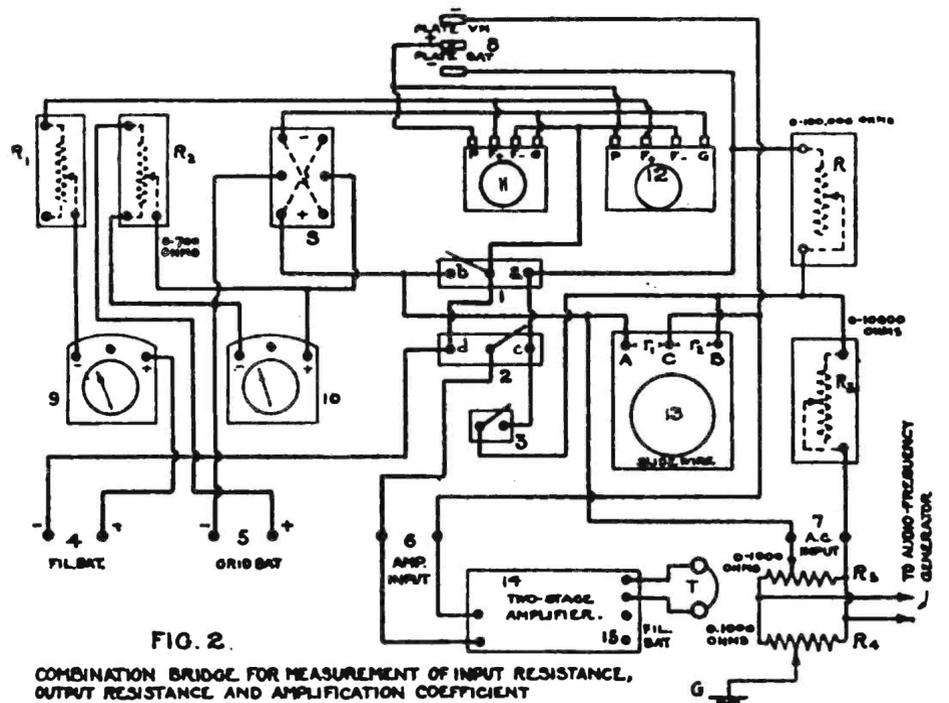
The slide wire and  $R_4$  are adjusted for minimum sound as described above and when silence is obtained
