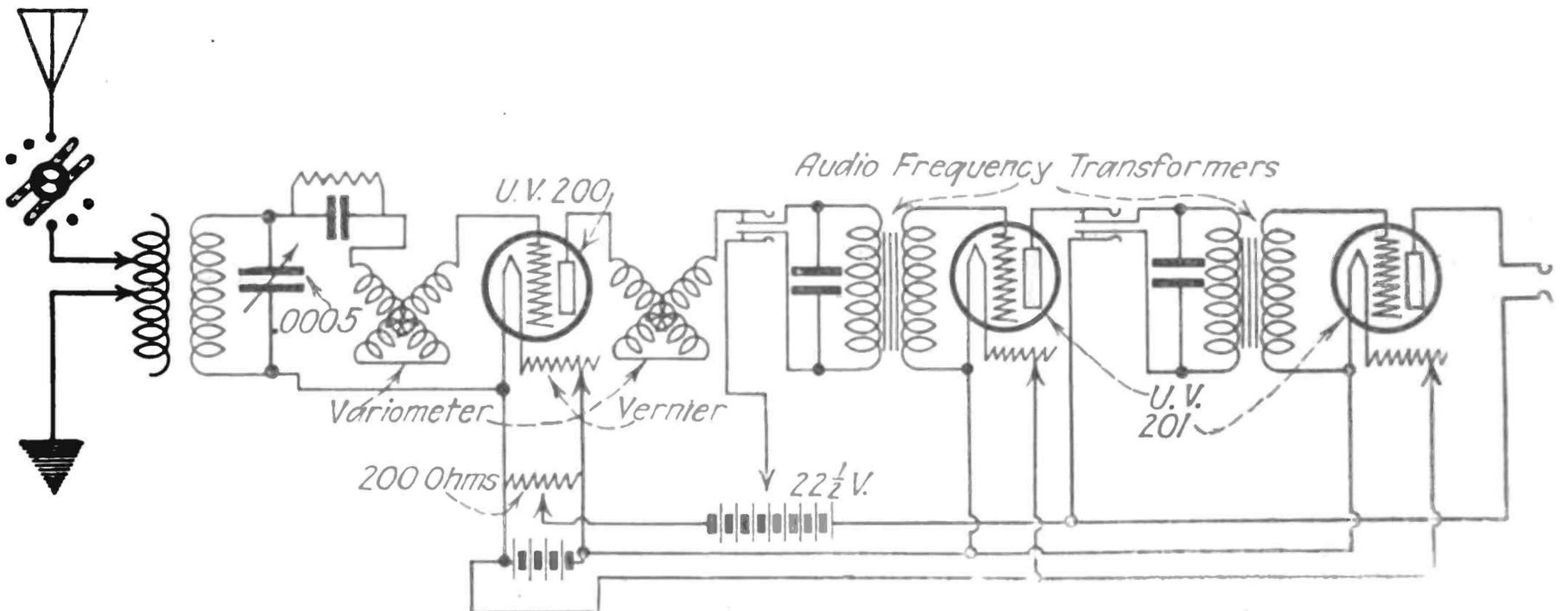
Hook-up furnished in response to query of Mr. G. W. Jamieson. It is the conventional regenerative hook-up embodying two variometers, a variocoupler and two steps of audio frequency amplification. The condensers across the primary of the transformers may be dispensed with if necessary, but, if used, will tend to decrease any tendency of the amplifier to howl and distort signals. The potentiometer should be 200-400 ohms resistance for most tubes.
