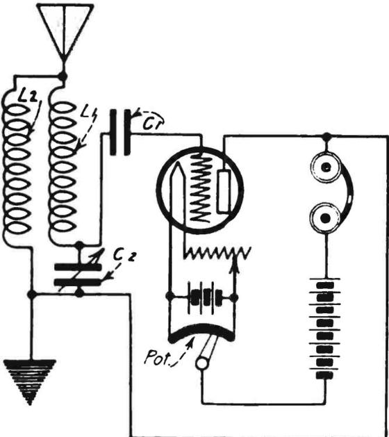
Fig. 3. Modification of Circuit 1. L1 can be a ... but must be placed in inductive ... C2, which is a coil of 175 turns.
