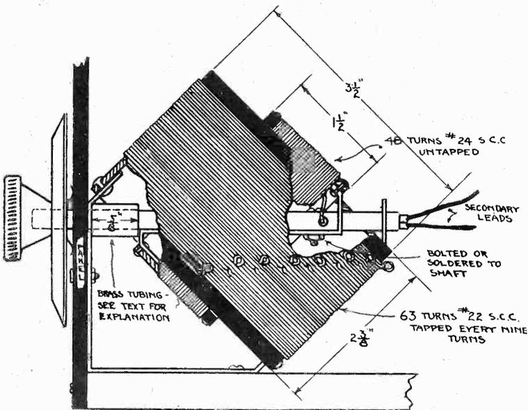
Fig. 1. Constructional details of the coupler described in the accompanying text. The secondary, or rotor, is fashioned to fit on a Z-shaped piece of metal allowing 180° variation, which is impossible with the present-day type.
