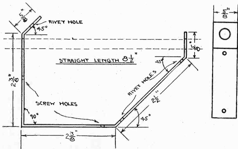
Fig. 2. The standard for the stationary coil is bent into shape from a strip of fairly heavy brass. It should be done very accurately if success is to be expected.
