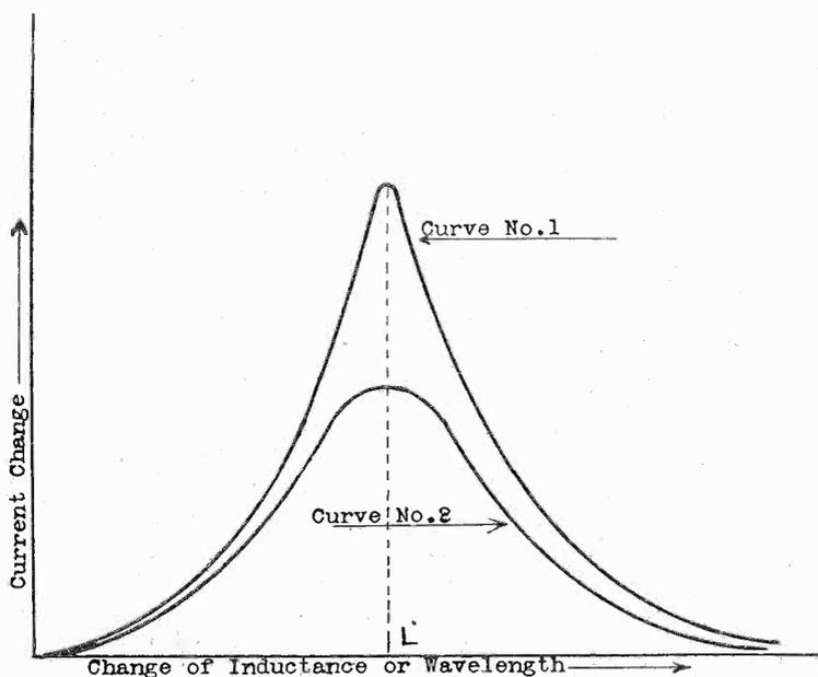
Fig. 2. Curve plotted to show current change as inductance is changed in the circuit.
