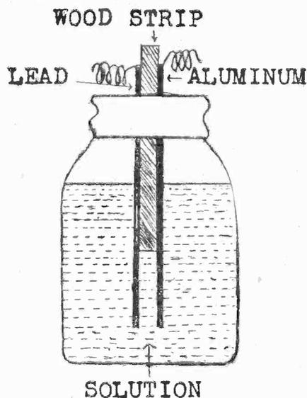
Fig. 1. Schematic drawing illustrating the method pursued in making up and arranging the elements of the rectifier.
