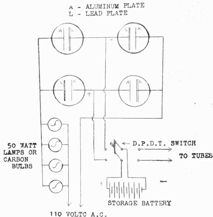
Fig. 2. Diagram showing how the rectifier should be hooked up, and also the method of connecting the series parallel bank of lamps.
