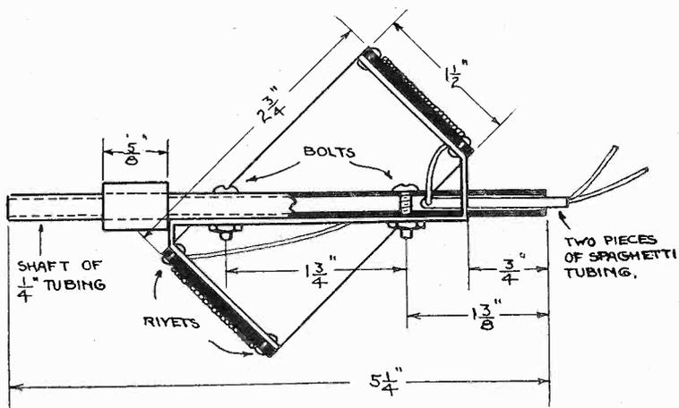
Fig. 4. Diagram showing the manner of fastening the coil on the standard. The shaft, which is hollow, is then bolted or soldered to the Z-shaped piece. This makes a solid looking and working rotor for the Ultimate Coupler.
