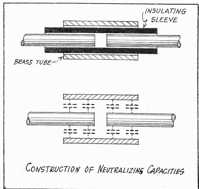
coupling between circuits is reduced to a minimum, if not to zero. The neutralizing capacity may have a capacitance of from 1 to 5 or 6 micro-micro-farads.
