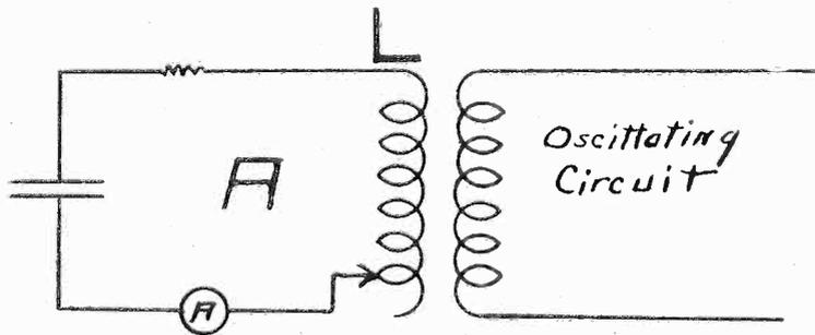
Fig. 1. Illustration depicting tuned primary circuit of a simple set, with ammeter in circuit to show current flow. This is the simplest type of oscillatory circuit.
