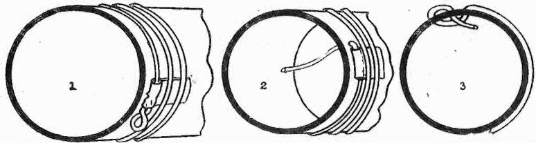
Fig. 5. Suggested method of fastening the first turn of the winding in order to prevent working loose. A strip of adhesive tape will do nicely.
