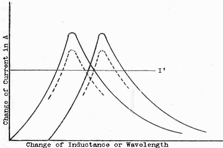
Fig. 5. Resonance curves representing two different waves corresponding to different stations sending at one time.
