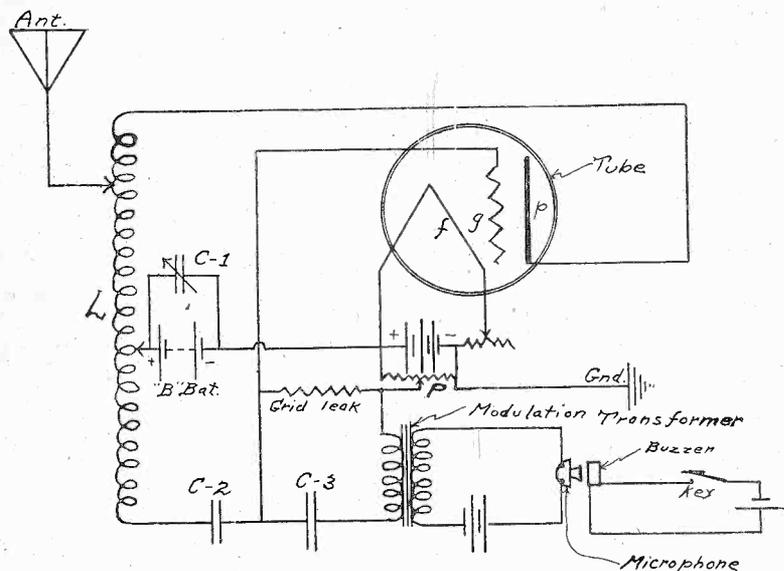
Diagram of the low power transmitter as described in the accompanying article. If the inductance L is constructed by the builder, extreme care should be taken in winding. Wire smaller than No. 22 should not be used. If a 5-watt tube is used larger wire should be used.
