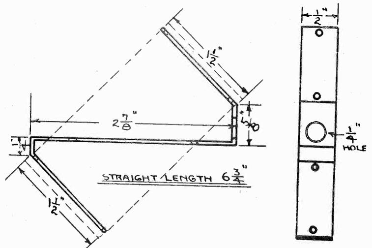
Fig. 3. The standard for the rotor which is bent out of heavy brass strip, and makes possible the 180° coupling.
