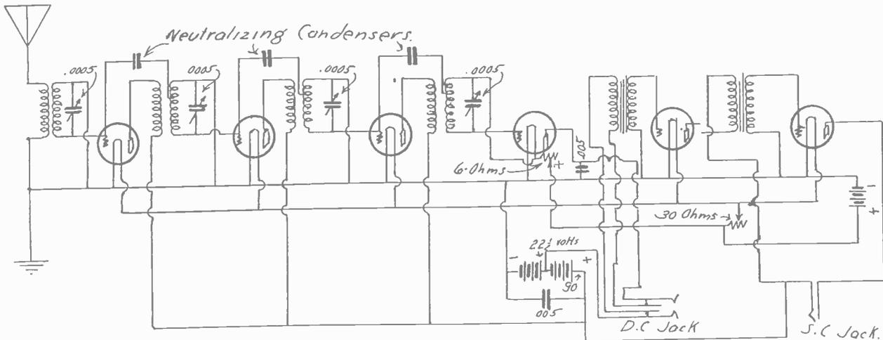
THE "SUPER SIX" NEUTRODYNE comprises three stages of RF, detector and two stages of AF.
