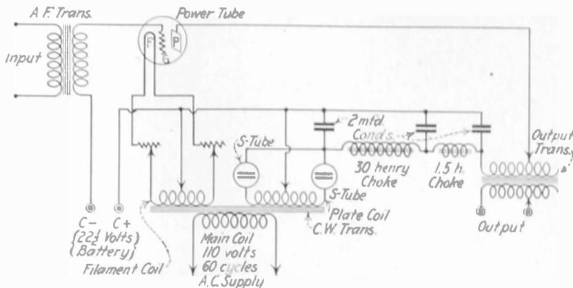
ONE TUBE power amplification, using filament transformer.
