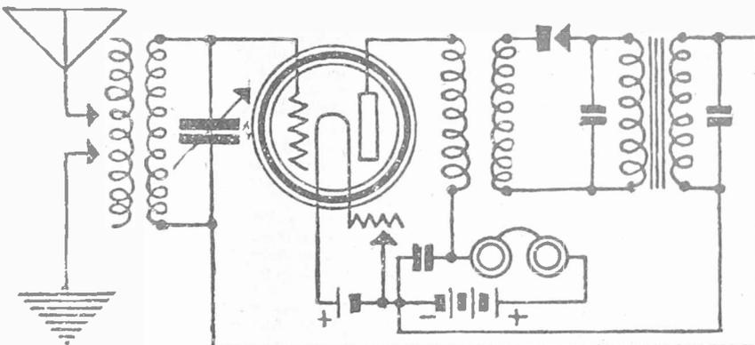
FIG. 5. Reflex circuit diagram asked for by J. O. Applegate
