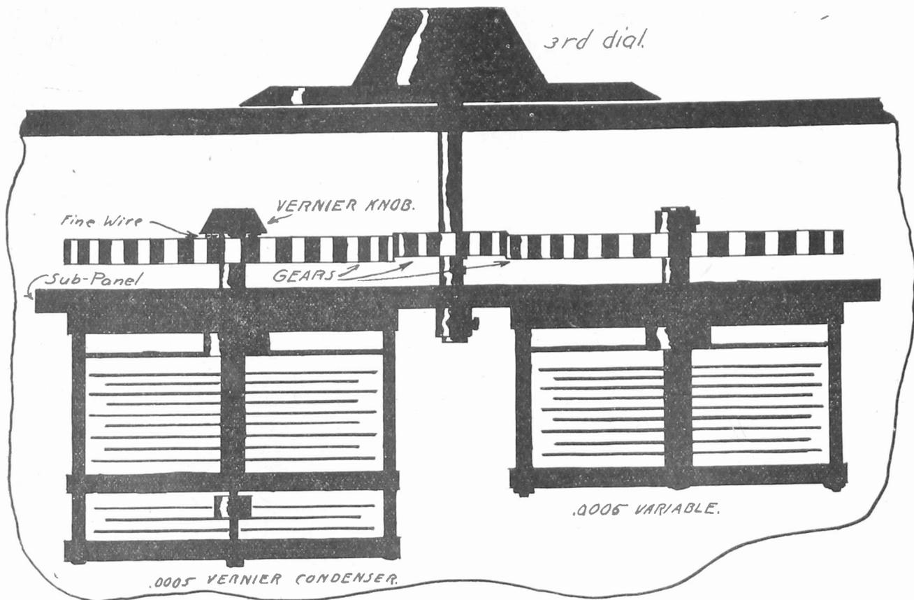
SO THAT ONLY THREE CONTROLS ARE NEEDED for a six-tube Neutrodyne, two condensers are tuned by a single knob, by gearing.
