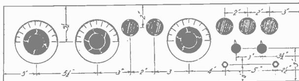
PANEL LAYOUT of Caldwell's "Super Six" Neutrodyne, showing the three dials that perfectly control operation, though an extra stage of tuned RF is added to the conventional five-tube set. The dimensions for drilling are shown in the illustration.
