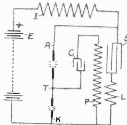
Means and apparatus used to produce sustained oscillations in a circuit.
