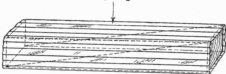
Fig. 2. Wood former used to wind the coils of the transformer. It is easier to wind it on the wood block than on the laminated leg.
