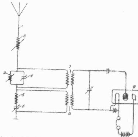
Circuit for the prevention of interference by means of double tuned inductances.
