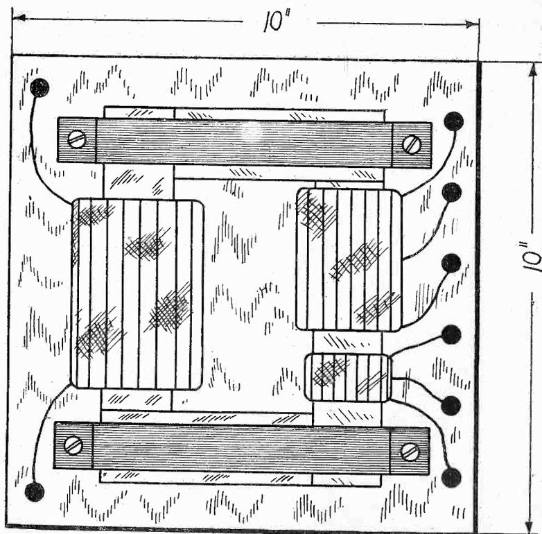
Fig. 4. Top view of the completed transformer showing location of binding posts and also the final placement of the coils.
