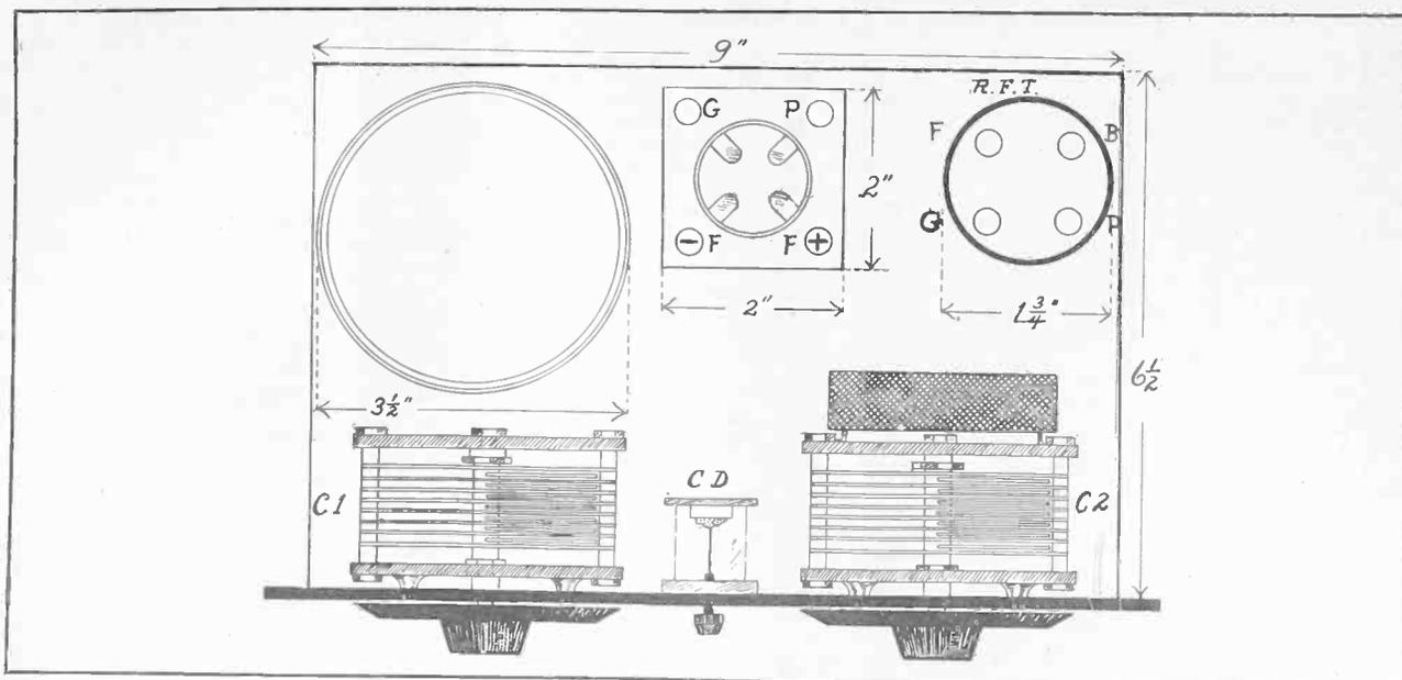
ASSEMBLY PLAN for the Bernard Superdyne (Fig. 3) showing the cylinder, at left, on which the coils  $L_1L_2$  are wound. The socket is in the middle and the iron-core radio-frequency transformer at right. The variable con-
