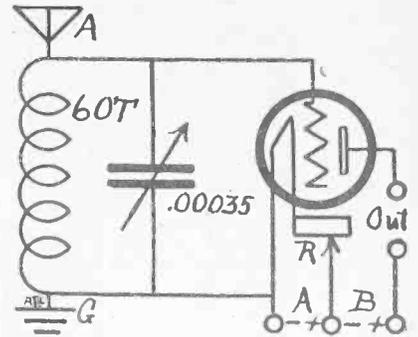
A STAGE of impedance-coupled radio-frequency amplification, which also builds up the audio signals somewhat. This works well ahead of the 3-circuit tuner.
