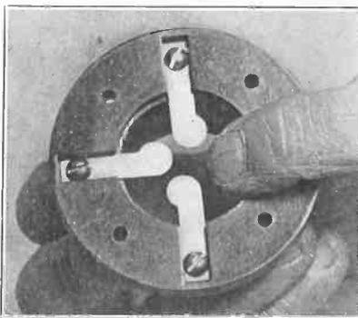
FIG. 3—The contacts of the vacuum tube socket forms the other half of the tube circuit. Placing a tube having clean prongs in a socket that has corroded contacts does little good. Both ends of the circuit must be electrically correct for best results.
