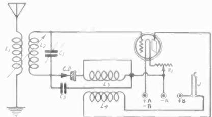
FIG. 5.—Circuit diagram of 2-control reflex that uses no audio-frequency transformer.
