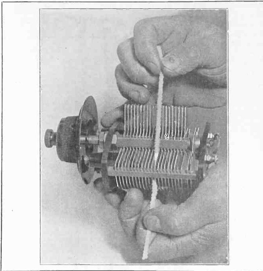
FIG. 4—The variable condenser plates must be kept clean. Dust between the plates causes noises, often mistaken for static. A pipe-cleaner saturated with alcohol will thoroughly clean the plates. However, it is necessary to dry the plates afterward with a fresh cleaner.
