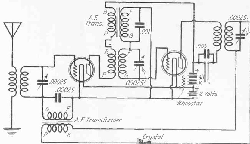
CIRCUIT DIAGRAM of Caldwell's 2-tube loudspeaker reflex.
