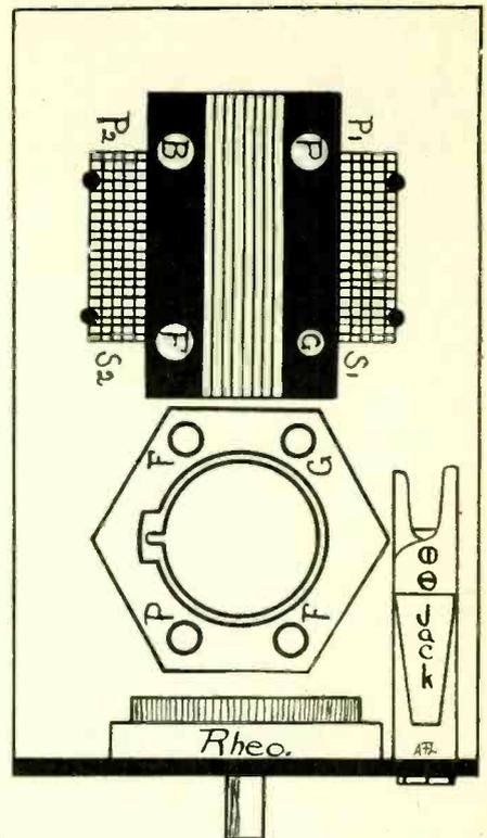
FIG. 2—Assembly plan of one stage of AF. The diagram is for 199 or 299 tube, but the text explains what to do if some other tube is used.
