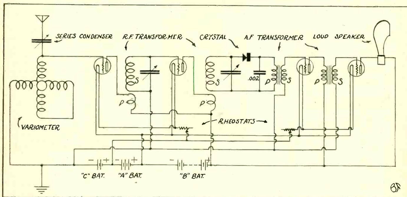
THE CIRCUIT is quite simple, with all unnecessary frills omitted. A C battery negatively biases the grids of all four amplifier tubes. The specially made primary windings of the RF transformers are marked P and the honeycomb coils S. Audio transformers are similarly lettered. This diagram reads from left to right, though the set is constructed right to left.
