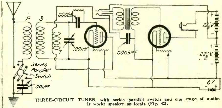
THREE-CIRCUIT TUNER, with series-parallel switch and one stage of audio. It works speaker on locals (Fig. 42).
