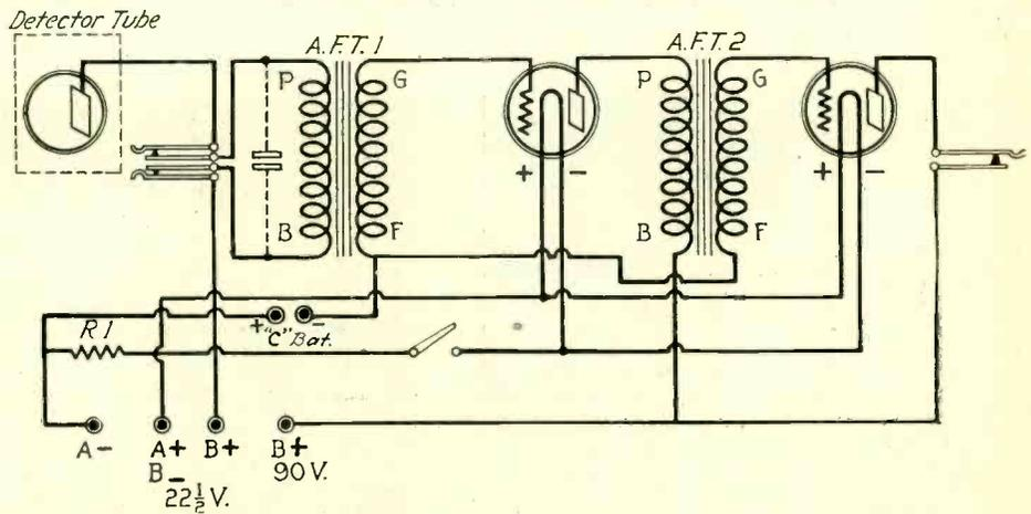
CIRCUIT DIAGRAM (Fig. 43) for two stages of audio-frequency amplification.
