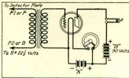
FIG. 1—Circuit diagram of one stage of transformer-coupled audio-frequency amplification. This is often enough to work locals on a speaker and makes DX reception more audible.
