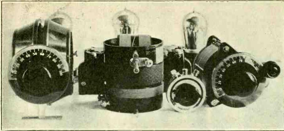
A VARIOMETER (at left) may be used for tuning the primary in a 3-circuit aperiodic set.
