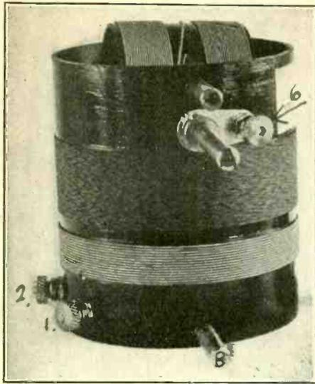
FIG. 3—A 3-circuit tuning coil, on familiar tubing, and not designed along low-loss lines, although a circuit in which it is used will function well. Binding posts, so far as shown, are numbered 1, 2 and 6, and the shafts A, B and C. How connections are made thereto is explained in the text.
