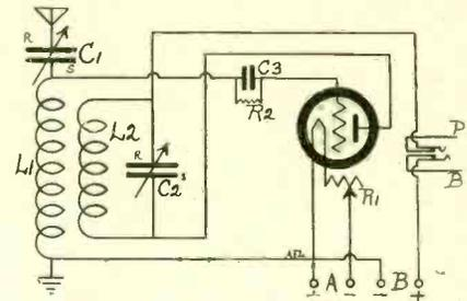
CAPACITATIVELY TUNED PLATE circuit affords fine control of regeneration. This circuit is splendid for those not living very close to a powerful radiocasting station, say 6 to 10 miles. It is fairly selective and has performed good DX work.
