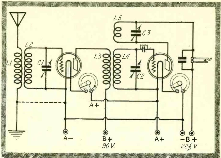
FIG. 1—Circuit diagram of a stage of RF ahead of the 3-circuit tuner.
