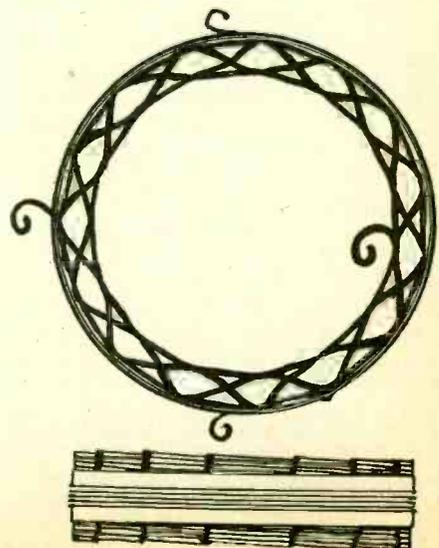
FIG. 3, top and side views of the completed RF transformer. The top view shows the terminals. The heavy zig-zag lines are the secondary. The circular lines on the outside are the primary.
