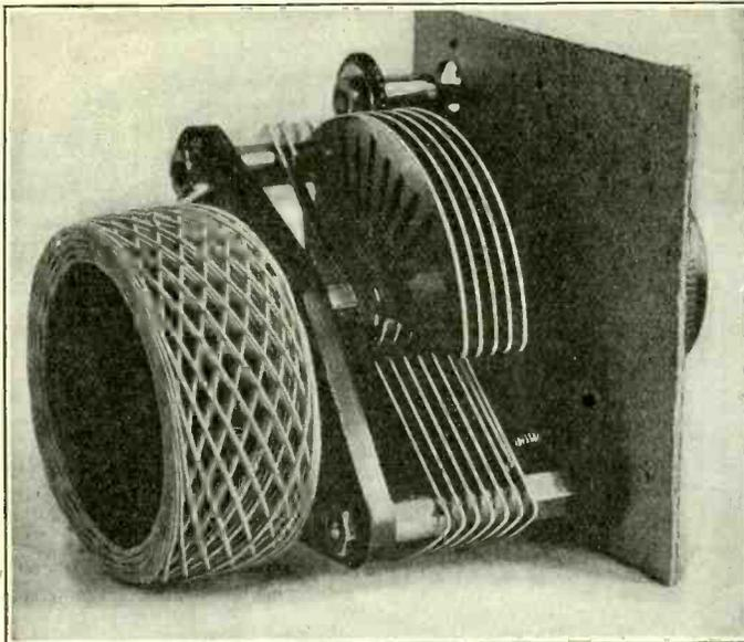
FOR A CONDENSER-TUNED PLATE a honeycomb coil may be used in this fashion, mounted on back of a variable condenser. If a 23-plate condenser is used the coil may be 50 turns. A duo-lateral coil and the spider-web described in text are of about equal efficiency.
