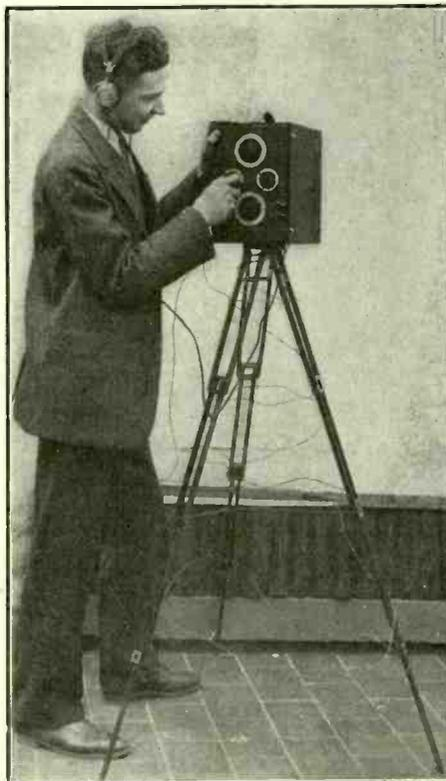
ON A TRIPOD, just like a camera, this radio set is mounted by a fan who goes on the roof to get best DX reception. The aerial hangs over the coping, as does the ground wire.
