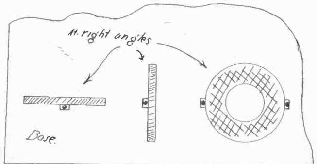
HOW the coils should be placed when mounted (Fig. 3.) They are at right angles to each other.
