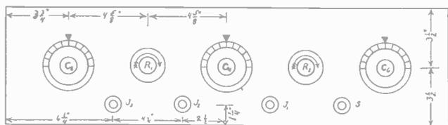
PANEL LAYOUT (Fig. 2) for J. E. Anderson's Simplified Neutrodyne.  $C_2$ ,  $C_4$  and  $C_6$  are the variable condensers for tuning. The dimensions for center shafts for drilling are marked on the diagram. The panel is 7 x 26 inches.  $J_1$ ,  $J_2$  and  $J_3$  are jacks and  $S$  is a switch.
