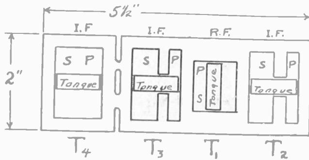
FIG. 6—Dimensions and shape of the components of the intermediate frequency transformers. These transformers pass side bands that bring the second harmonics through the loud speaker for quality reception of music. The transformers are designated to correspond with the lettering in the circuit diagram on page 6.
