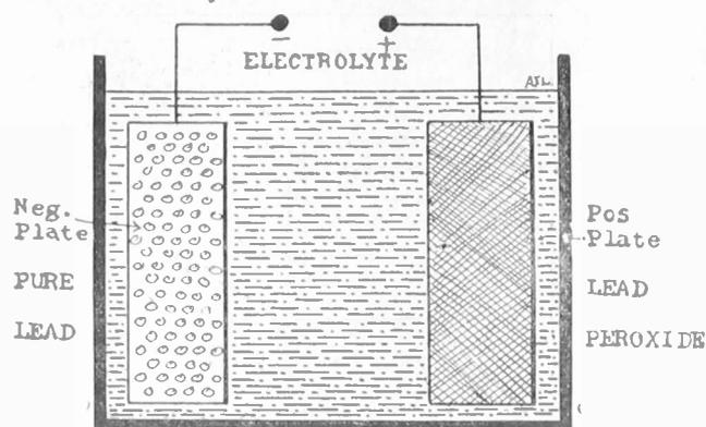
FIG. 1, storage battery cell. When the battery is charged the negative plate becomes spongy and the positive plate becomes covered with a coating of lead peroxide. The 20% solution of sulphuric acid should cover the top of the plates.
