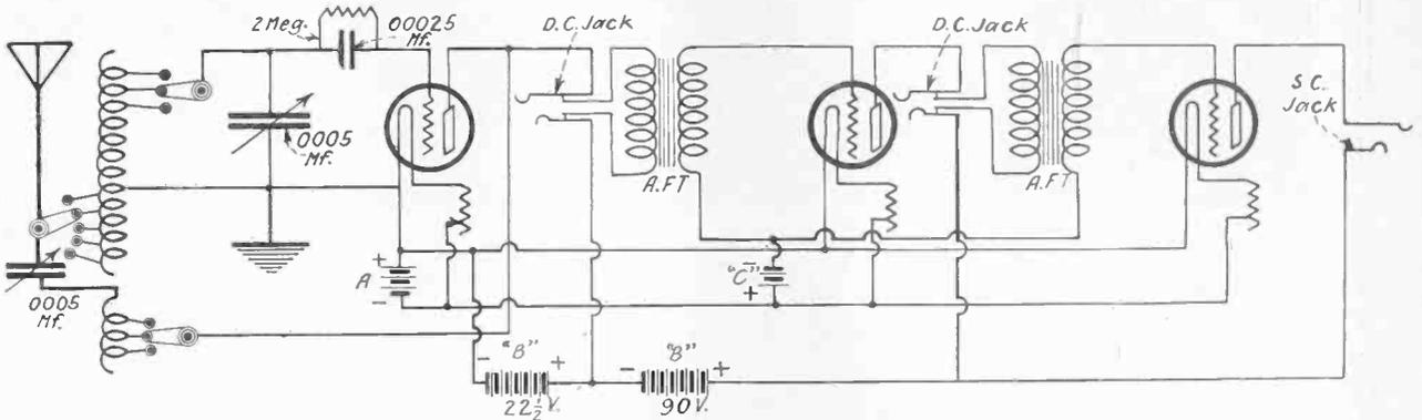
FIG. 32—Reinartz hook-up with two stages of AF amplification. One 4 1/2-volt C battery is used for both audio stages. Excellent loud speaker volume may be had from local and distant stations with this circuit.
