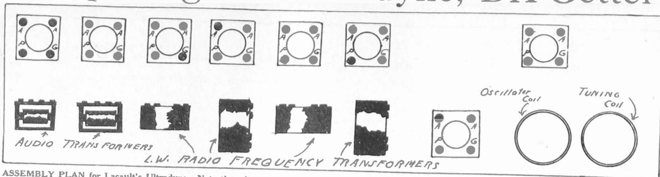
ASSEMBLY PLAN for Lacault's Ultradyne. Note that the tuning and oscillator coils are at right, the two AF transformers at left. Between are the intermediate frequency transformers and all the sockets except the two for the first detector tube and the oscillator tube. This arrangement makes for neatness and efficiency.
