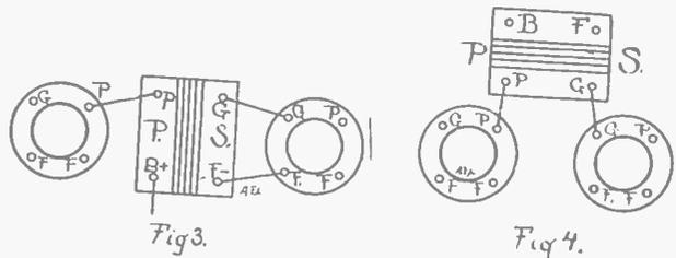
HOW to use a depth gauge is shown in Fig. 1. Two ways of placing the AF transformers are represented in Figs. 3 and 4, while Fig. 2 shows how to measure distances between holes. Fig. 2 is the small template under Fig. 1.
