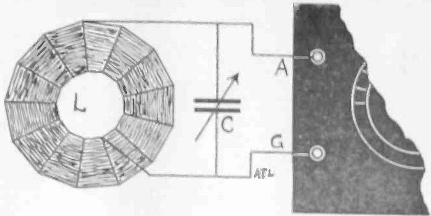
HOW to connect the coil and condenser of the wave trap in your receiver. The coil may be a spider-web, as shown, or a 50-turn honeycomb and the condenser a 23-plate variable. The wave trap is effective when located at a fair distance from powerful radiocasting stations.
