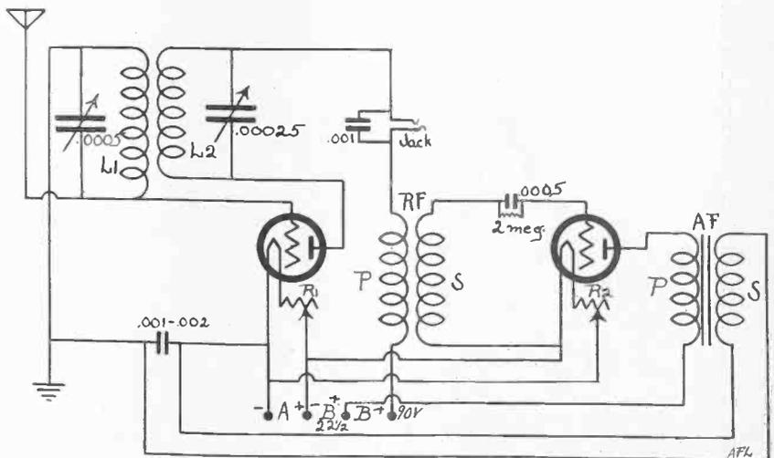
FIG. 31, hook-up of the 2-tube reflex asked for by H. T. Hadden, Bluefield, W. Va. There are two tuning controls, one for the first tube at radio frequency, and the other for the detector tube. The signal is reflexed back into the first tube and amplified at audio-frequency.
