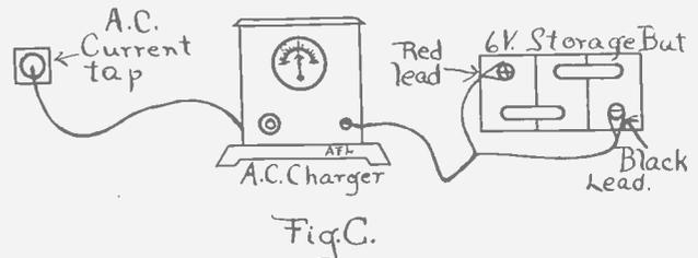
FIG. 3C—Alternating current charging device which works on the magnetic rectification principle. With this type of charger the battery is left on the line about 24 hours in most cases.
