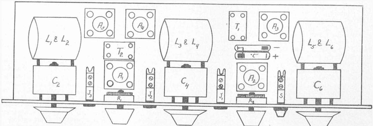
ASSEMBLY LAYOUT for the simplified neutrodyne. The wide spacing of the tuned radio frequency transformers prevents intercircuit oscillation. The C battery has a total of nine volts which is necessary for the amplifier grid bias when more than 67½ volts are used on the AF tubes. The AF transformers are also widely spaced. The binding posts may be mounted on a bakelite strip at the rear of the baseboard.
