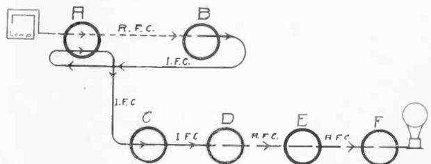
FIG. 2—The path of the signal in the new Super-Heterodyne. A, B, C, D, E and F are the tubes. R.F.C. is RF current and I.F.C. is intermediate frequency current. E and F handle AF current.
