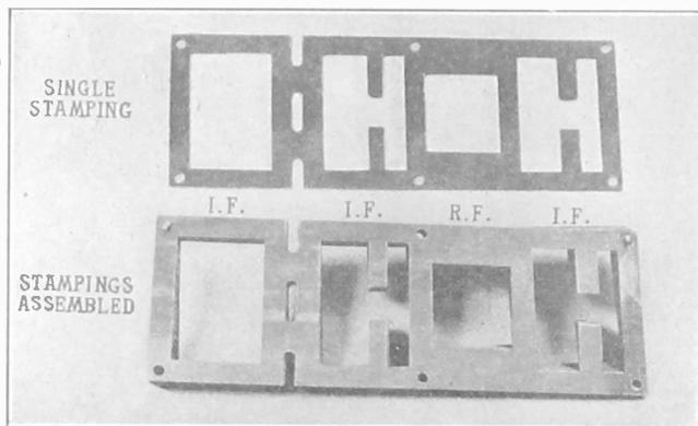
FIG. 7—Stampings used in the construction of the intermediate transformers. These transformers represent an engineering feat and the details of their construction are herewith presented for the first time.
