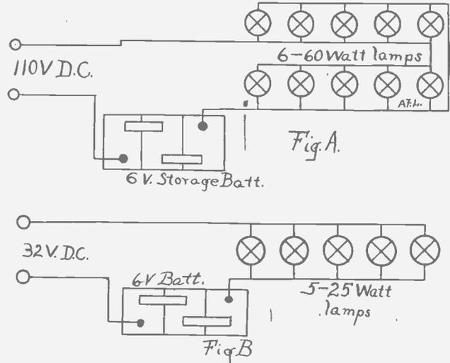
FIG. 3A—Circuit for charging the battery at home off a 110-volt direct current line. After 12 hours on the line one bulb is taken out, and one each 2 hours thereafter. This reduces the charging rate. Altogether the battery should stay on the line about 20 hours. Fig. 3B is almost identical except that it is for charging the battery on a 32-volt farm lighting generator. Always put positive to positive and negative to negative when charging.
