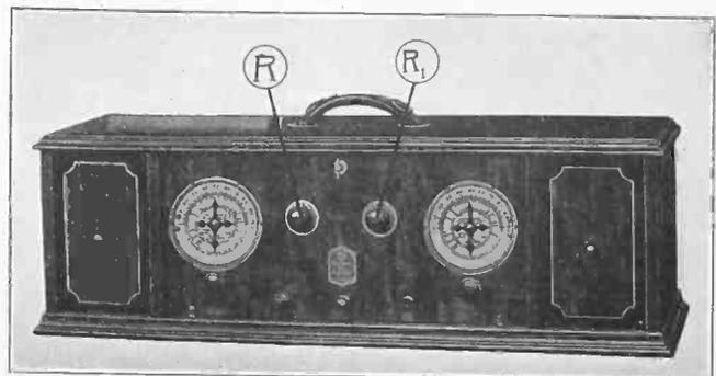
FIG. 3—Front view of the set. R and R1 are rheostats.
