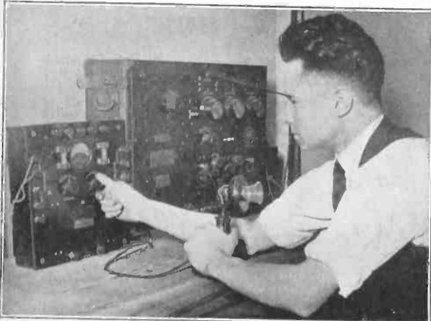
TESTING the new type Signal Corps radio telegraph and telephone outfit. The meters tell when the set is radiating best.
