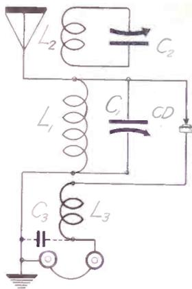
FIG. 3A—How a 3-circuit tuning coil may be employed in a wavetrapped crystal hook-up. L1 is the rotary coil. L2 is the secondary (large stator winding, used for trap). L3 is the otherwise aperiodic primary. The rotary coil L1 is loosely coupled and left that way.
