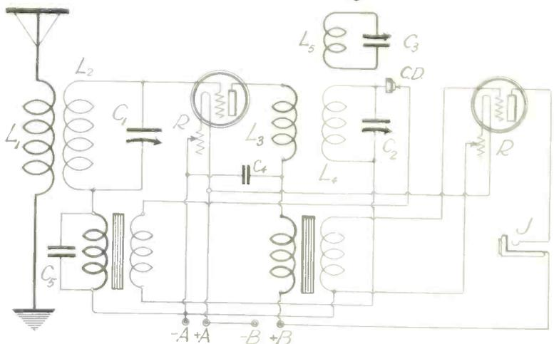
**ONE STEP FARTHER** and we have a reflex set that works a loud speaker and which is selective. The wave trap idea is retained. This is the same as Fig. 4, except that a second stage of audio (this one not reflexed) is added. (Fig. 5.)
