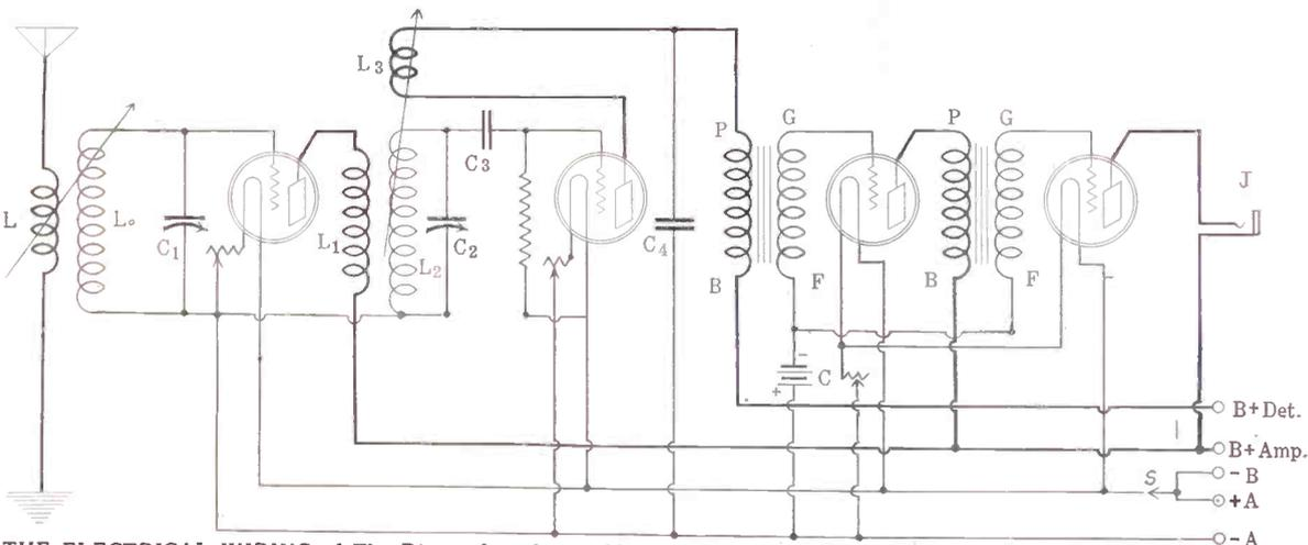
THE ELECTRICAL WIRING of The Diamond, with variable antenna coupling (Fig. 185). L may be the tickler of a vario-coupler, L0 a secondary made to match the condenser C1. The set will have four controls, unless C1C2 is a double condenser, whereupon there are three controls. L need be varied only occasionally, hence the set would be practically in the 2-control class. Constants are given in the May 23 and July 25 issues of RADIO WORLD.
