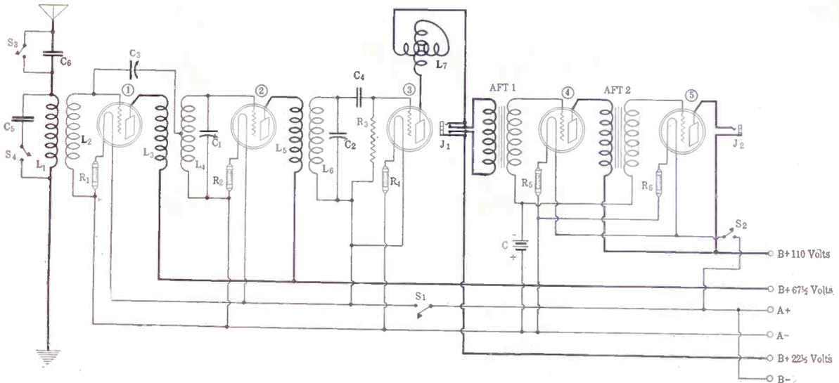
Fig. 1, showing the electrical diagram of the Improved Diamond. There are 5 tubes in this set instead of 4 tubes as in the original Diamond.
