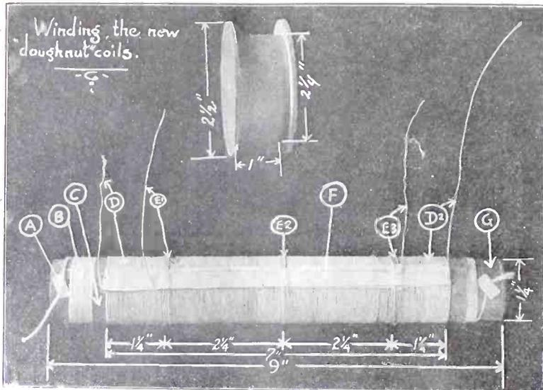
FIG. 1, showing (on top) the spool which constitutes the mount or form on which the coil is placed after being wound, and (lower view) the original form on which the wire is placed prior to removal. The text explains the designations. The completed coil (Fig. 2) is shown on the front cover.
