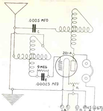
FIG. 189, showing a receiver employing 1-Tube, the grid and plate being tuned by variometers. The rheostat has a resistance of 10 ohms. When building this set, place the variometers no more than 2 3/4" away from each other. The mid-tap is taken where the rotor and the stator join.
