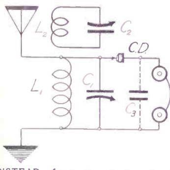
INSTEAD of two wave traps one may be used, but that is efficient only if the receiver has a 2-station range. (Fig. 3.)
