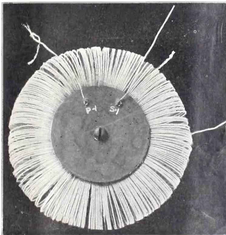
The Completed Toroidal RF Transformer. (See page 6.)
