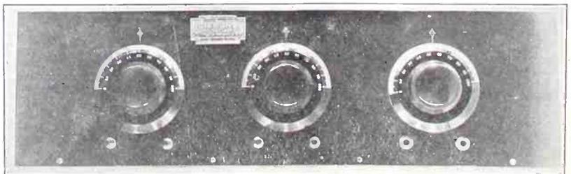
FIG. 4, showing the front panel view of the set. The first dial controls the shaft of the variable condenser shunted across the second RFT and the other dial controls the shaft of the condenser shunted across the secondary of the detector coil. The other dial controls the rotor of the variometer.
