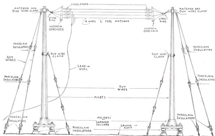
MANY folks think an antenna having four wires improves the reception of signals. This type of antenna causes very broad tuning, due to the large amount of capacity and effective antenna resistance. A great many of the present day transmitters desire a lot of capacity, due to the high power. In the transmitter the resistance is overcome by the high voltage output, but in the receiver, there is no output it is all coming in and nothing to counteract this resistance. With an antenna the multi-
