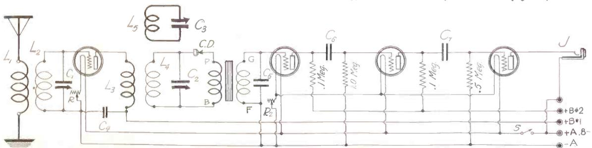
THE SAME CIRCUIT as shown in Fig. 6, except that the first audio stage is not reflexed. (Fig. 7.)
