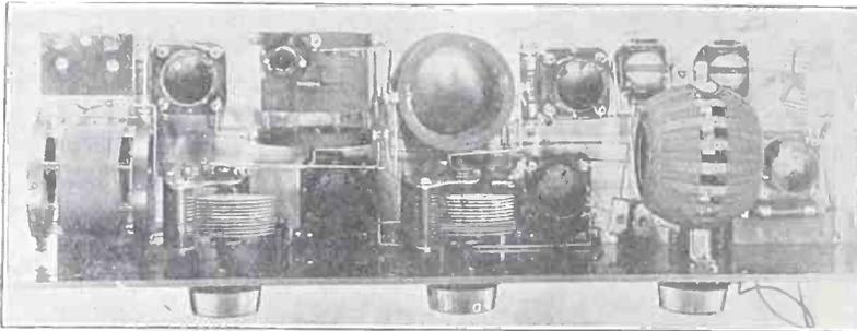
FIG. 3, looking down on the receiver. This photo gives a good idea of how the parts should be placed on the baseboard.
