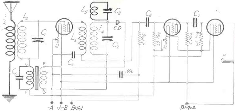
THE SAME fundamental hook-up as is shown in Fig. 5 is presented above, except that the second audio stage is replaced by two stages of resistance-coupled AF for better quality. (Fig. 6.)
