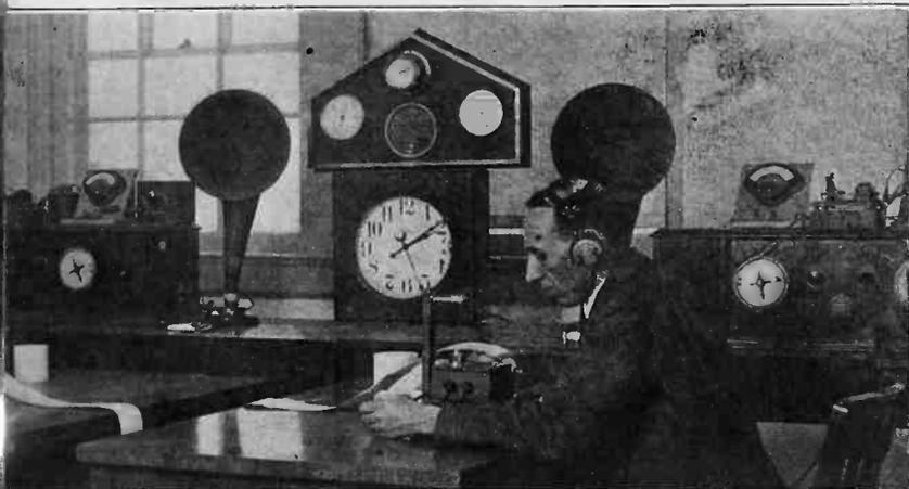
of America used in observing the action of the sun on radio waves, during the total eclipse of the sun. er for longer wavelengths. It was found that the sun greatly interfered with reception on short waves, ng waves. The photo shows A. Van Dyck, division engineer of the R. C. A.; Dr. A. N. Goldsmith, b engineer. They are making tests on the "fading recorder." (Wide World).
