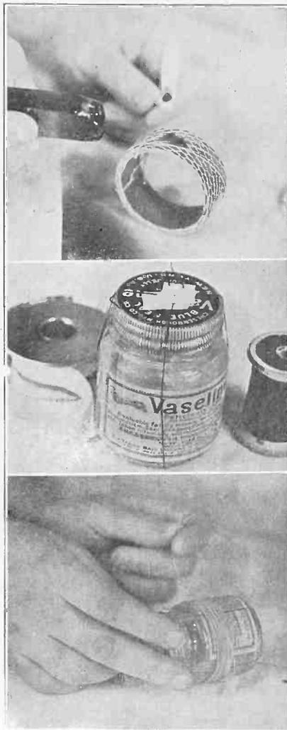
FIG. 2 (top) shows how sealing wax is used to bind the new end of the coil. The middle photograph (Fig. 3) shows how two pieces of thread wound the length of a small vaseline bottle and secured on top with adhesive tape. The roll of tape is at left. At right is the spool of thread. Fig. 4 (bottom) reveals the method of winding the excess wire, taken from the honeycomb coil, right on the vaseline bottle.
