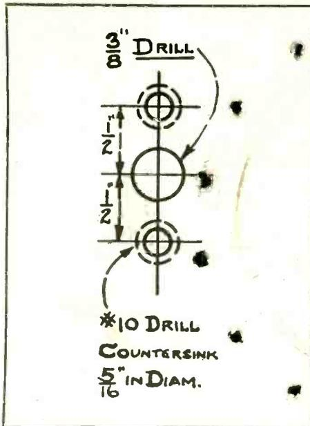
FIG. 6 template for drilling holes in the panel for mounting the special variable condenser used in the Superdyne. The center hole is for the condenser shaft and should afford free clearance. The two other holes are for the mounting screws.
