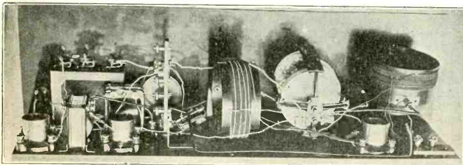
FIG. 7, rear view of the interior. The coupler is at right, the variable condenser next to it, then the radio-frequency transformer, which is tuned by the same variable condenser that tunes the coupler secondary. (RADIO WORLD staff photo.)
