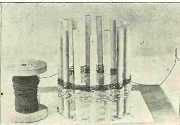
FIG. 9—The beginning of the primary winding, after the sixteenth turn of the secondary. The primary, consisting of twelve turns, may be completed before the winding of the secondary is resumed. Both windings should be in the same direction. For temporarily securing the wire terminals they may be looped around a dowel.
