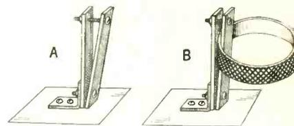
**FIG. 73**, how to mount a honeycomb coil on the baseboard. Two strips of bakelite or seasoned wood act as a vise, adjustable by two screws. Screw the strips to the wood baseboard. If no baseboard is used, the entire instrument may be mounted similarly on the back of the panel.
