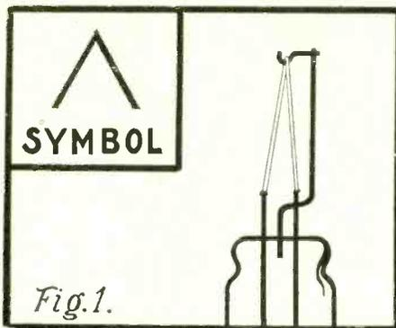
THE FILAMENT is symbolized by an inverted V or U. At right is a graphic representation of the filament, a key to the origin of the symbol.
