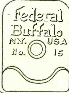
Moulded bakelite shell of two pieces totally enclosing terminals and affording operator a firm, yet convenient, grip.
