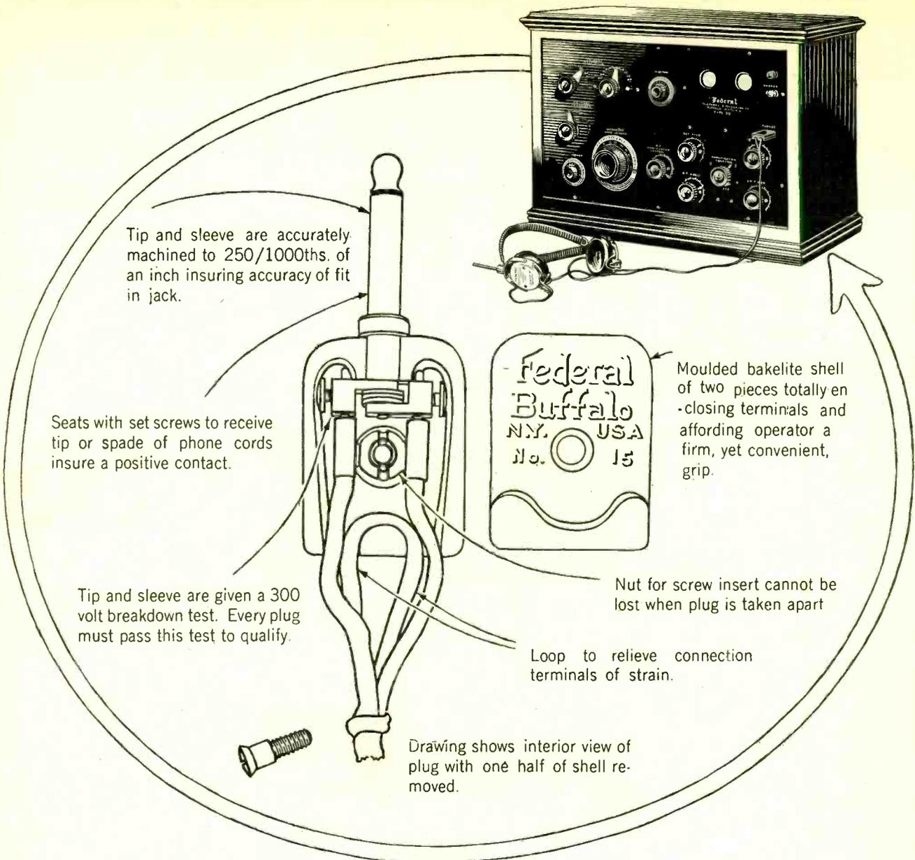
Tip and sleeve are accurately machined to 250/1000ths. of an inch insuring accuracy of fit in jack.
