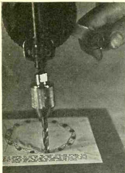
FIG. 5—Showing wrong way to drill.
