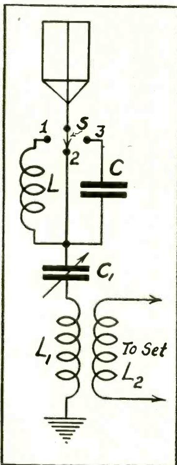
FIG. 2, showing the aerial and ground at top and bottom respectively. L, L1 and L2 are coils, represented by series of loops. A condenser is shown by two parallel lines (C), while, if variable, an arrow intersects the symbol. This diagram shows how to use a loading coil L and fixed series condenser C for varying the aerial's wavelength electrically.
