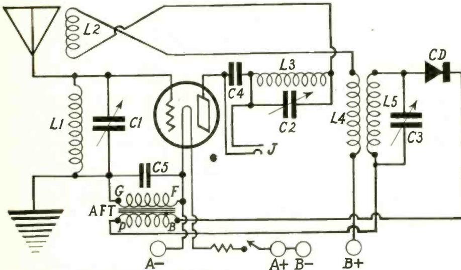
THE 1-TUBE Reflexed Superdynamo diagrammed above, affords fine signal quality because of the crystal used as the rectifier. This circuit is not selective enough for those living in cities. L1L2 are both on one tubing and are fixed coupled. All the coils may be made at home. There are three controls, the variable condensers C1, C2 and C3. This is a good reflex for the beginner to build. It is not a DX set. The circuit was described in the December 6 issue.
