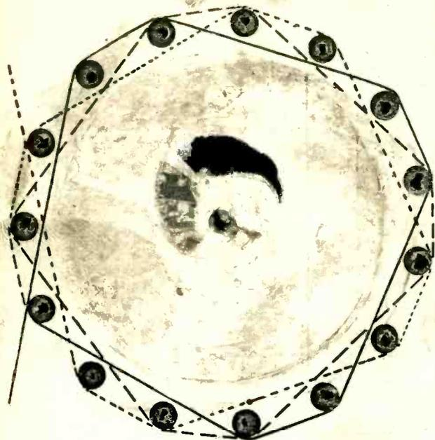
FIG. 2—Template for making the wooden block and inserting dowel rods to wind the low-loss coil. The rods are inserted in drilled holes and are at right angles to the base. The wire is wound in and out of alternate pairs of rods. The solid line represents one turn, the dotted line the next turn and the dash line the next. The coil is made self-supporting. The diameter between dowel centers is 3 inches.
