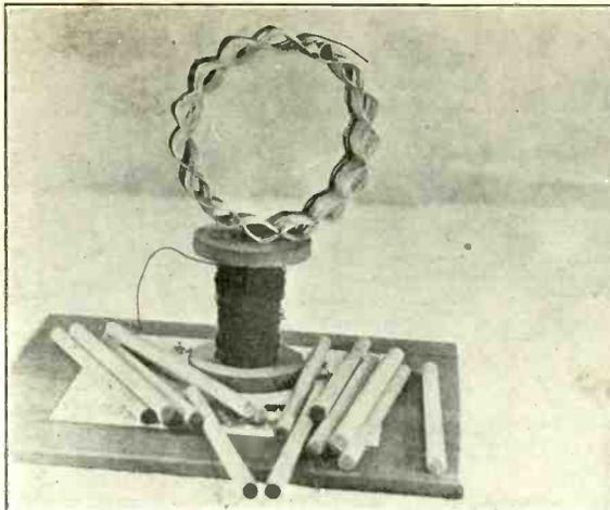
FIG. 6—An anticipatory glimpse, showing what the completed coil will look like, and revealing the spool of primary wire, dowels and block with template pasted on it. Note that on this particular coil an aperiodic primary has been wound of dark-covered wire, to distinguish it from the white-covered secondary.
