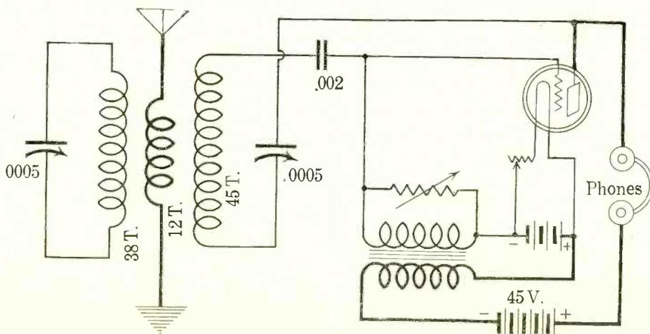
AN ULTRA-Audion Reflex, the design of which was submitted by Seeley Hopkins, 2416 Madison Avenue, Ogden, Utah. A variable resistance is used across the transformer secondary. This is a leak. The three coils are on a  $3\frac{1}{2}$ " diameter tubing, 6" long, in the order shown in diagram, or the absorption coil may be on a separate tubing, inductively coupled to the other coils. No. 22 SCC wire may be used.
