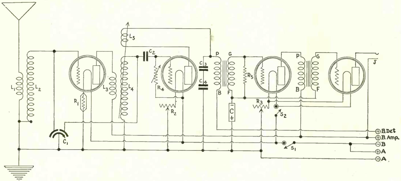
THE circuit diagram of the 2-control Diamond of the Air as used by Capt. O'Rourke on a motorboat. C1 is the double condenser. The construction was described by Herman Bernard in the May 23 issue. C3 and C4 are helpful, but not vital. Try them in both positions shown in diagrams
