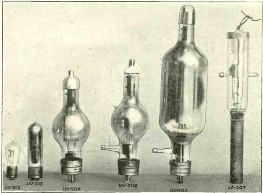
FIG. 3, showing the six different sizes of tubes used in commercial and amateur circles. The UV202 is the 5-watt, UV203 is a 50-watt (old style, filament ampeers, 6.50); UV204, a 250-watt; UV206, a 1,000-watt tube; UV208, a 5,000-watt tube. The UV207 is a water-cooled tube, with an output of 20 kilowatts.
