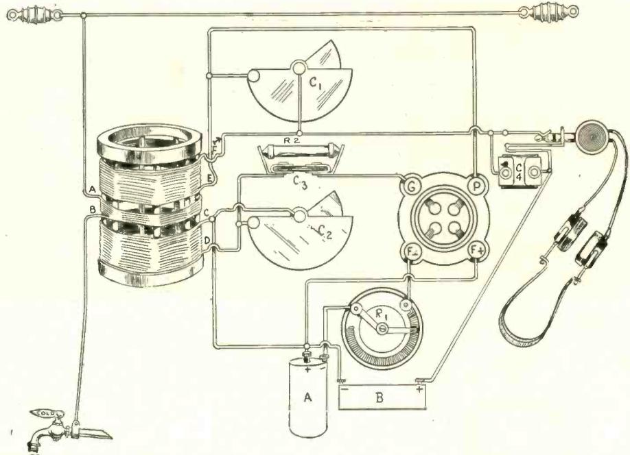
FIG. 168, showing the picture diagram of a 1-tube DX set. The tubing is 3" in diameter and 4" length. There are 50 turns on the grid coil (C and D), 10 turns for the primary coil (A and B), and 35 turns for the plate coil (E and F). Leave 1/2" spacing between coils. The variable condensers (C2 and C3) have a maximum capacity of .0005 mfd. The coil wire is No. 22 SCC. Keep the polarities in the same manner that they are shown on diagram. Use a WD12 tube for the detector and a 6-ohm rheostat.
