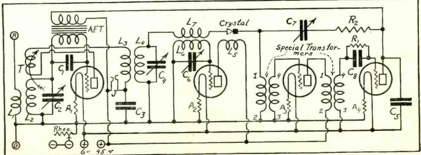
THE WIRING of the 4-tube Baby Super-Heterodyne. For simplicity the reflex stage should be avoided, although the more experienced will fare very handsomely on the 4-tube basis.
