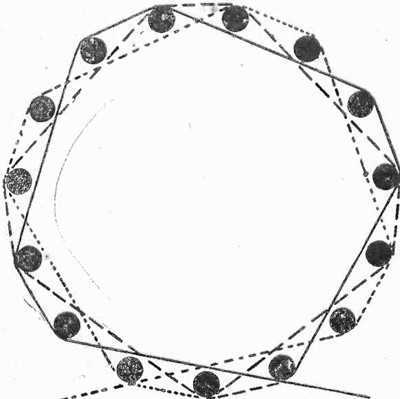
FIG. 2, template for basket-weave form. Take a 4" square block of wood, drill 3/16" holes as shown. Insert 3/16" dowel sticks, each cut to 4" length. These are at right angles to the wooden base. The sticks may be glued in place. Using No. 18 DCC wire, wind under two turns, over two, under two, over two, etc. Right to left, the solid line represents the first turn, the dotted line the second, the dash line the third.
