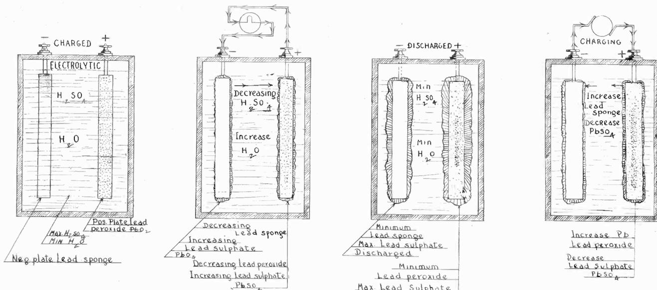
Fig. 1—The picture tells the story. In the last diagram "Pb" should read "PbO<sub>2</sub>." In the extreme left-hand diagram the solution called electrolytic should be electrolyte.
