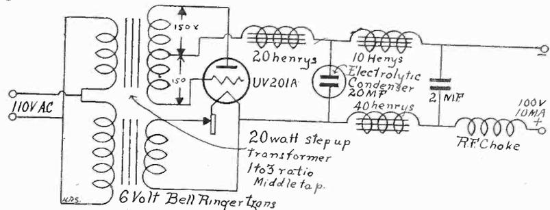
FIG. 3—Using a 6-volt bell-ringing transformer and a UV201A to step-up and rectify AC for use on plate of amplifier tubes.
