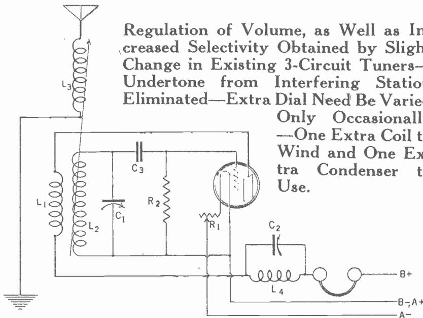
**Regulation of Volume, as Well as Increased Selectivity Obtained by Slight Change in Existing 3-Circuit Tuners—Undertone from Interfering Station Eliminated—Extra Dial Need Be Varied Only Occasionally—One Extra Coil to Wind and One Extra Condenser to Use.**
