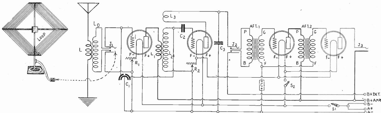
FIG. 1—The wiring diagram of The Diamond of the Air as a 2-control set, with option of loop or aerial operation. L0 and L2 must be matched; and the loop must be matched with them, too. Various methods of accomplishing such matching are discussed in the text.
