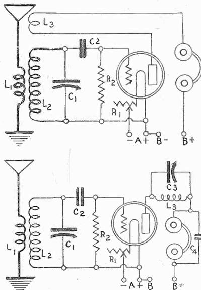
FIG. 1, top, the inductive tickler regenerative set, known as the 3-circuit tuner, employing aperiodic primary. This hookup works well on short-wave work, as does the other, Fig. 2, which embodies a fixed coil in the plate circuit. This plate coil, L3, is tuned by a variable condenser to obtain regeneration through the internal capacity of the tube.
