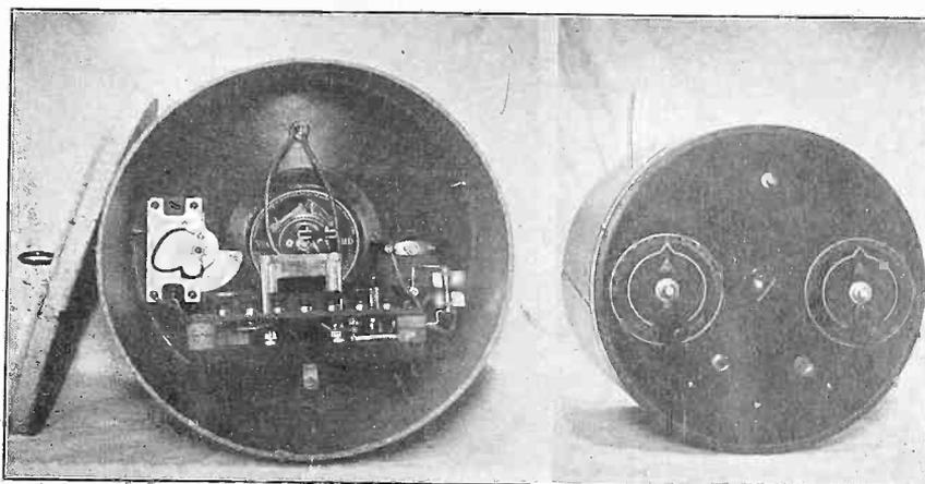
USING a phonograph record as a panel for a portable radio set the result is shown above. The material in the record is a very good insulator. Note the space inside for batteries. (Kadel & Herbert)
