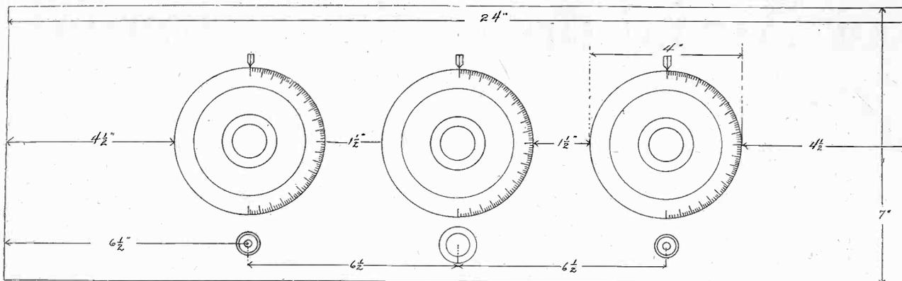
FIG. 3—Front panel layout of the Low-Loss Neutrodyne. The switch may be inserted in the left-hand corner or right-hand corner of the panel.
