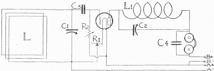
FIG. 3—A 1-tube loop set that brings in local stations. The range is about 50 miles, often much more. It is a good circuit to use to calibrate C1 as against inductance L, which is the loop. C2 is .0005 mfd., L1 is 45 turns of No. 20 DCC wire on a 3½-inch diameter. C4 is .002.
