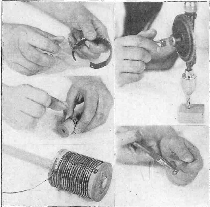
FIG. 1, top left, removing resistance wire from an old rheostat. Fig. 2, on an ordinary spool wind this wire. The completed winding is shown in Fig. 3, bottom left. Cut a block of wood 1" thick and 2" square (Fig. 4, top right). Drill a 1/4" hole, to insert a dowel stick, take an old switch arm, bend it back a little. See Fig. 5. (Hayden).
