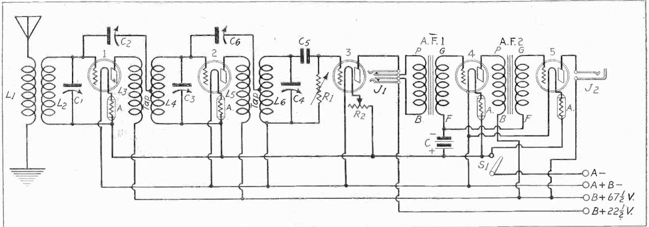
FIG. 1, the circuit wiring of the Low-Loss Neutrodyne. The coils L1L2, L3L4 and L5L6 are basket-weave. The neutralizing condensers are C2 and C6. A C battery is used to bias the audio tube grids. S1 is a master switch, push-pull or toggle. One rheostat is used (R2 in the detector circuit). A represents ballast resistances. They, like the rheostat, should be in the negative A battery lead, as shown.
