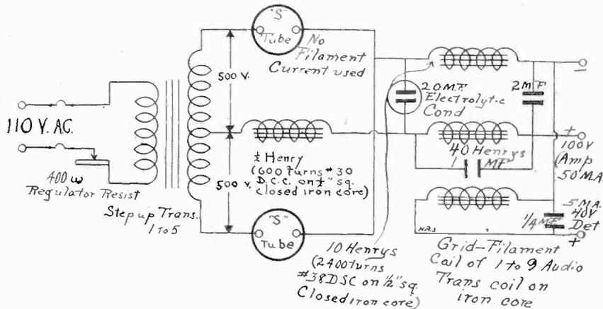
FIG. 2—How to use S tubes in the rectifier unit.
