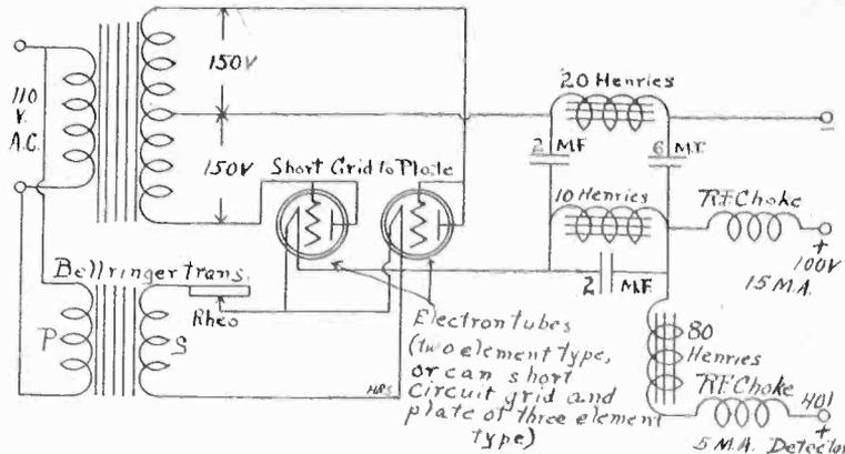
FIG. 1—The UV201As come into excellent use here for rectifying the AC for supplying B battery potential.
