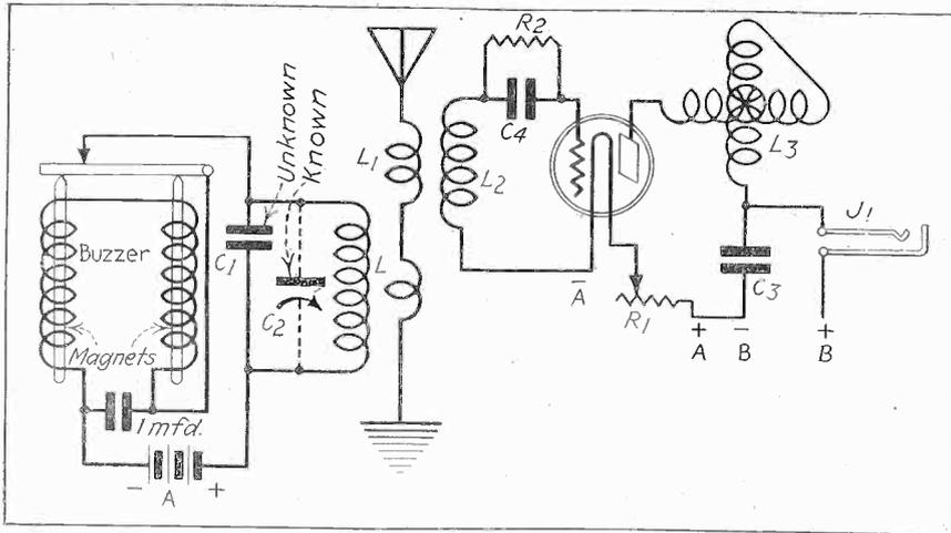
FIG. 1, showing how the unknown capacity of a condenser (fixed or variable) is determined by the wavemeter test.  $L_1$  is the regular aperiodic primary of a receiver and  $L_2$  a small extra winding (6 or 8 turns) in inductive relationship to the wavemeter coil next to it. No variable condenser is needed on the receiver.
