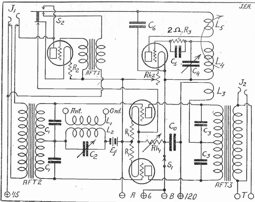
FIG. 1, schematic wiring diagram of J. E. Anderson's Twinplex, where push-pull AF is used for fine quality with great volume. The RF stage is in parallel, being reflexed in the push-pull stages, Mr. Anderson's original idea.
