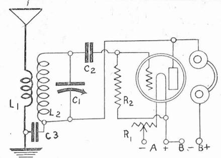
FIG. 136, the 1-tube, 1-dial DX set. L1 is the primary while L2 is the secondary, both of which can be wound on a 3 1/2" tubing, 4" high, using No. 22 DCC. L1 consists of 12 turns and L2 of 47 turns. C is a .0005 variable condenser. The regeneration is controlled mainly by the rheostat. C2 is the .00025 mfd. grid condenser, C3 is .001 mfd. This set works well on dry-cell tubes.
