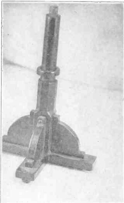
FIG. 1—Close-up of the stand. This measures about 6" high and has been turned from a piece of wood 1" diameter. The little feet, four of which are used, extend out from the sides of the main upright about 2½". Notice the top of the stick which has been turned down to about ½" diameter. This fits into the base of the loop. This is an elaborate device and the same practical effect can be attained by using a ½" dowel stick and an ordinary loop base.
