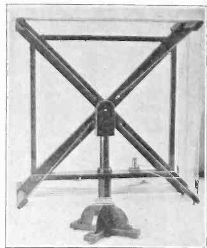
FIG. 5—A view of the completed loop. The type is referred to as box loop. It measures 12" square. A ½" hole has been drilled in the center-piece so that the stand fits in and allows the loop to be turned freely
