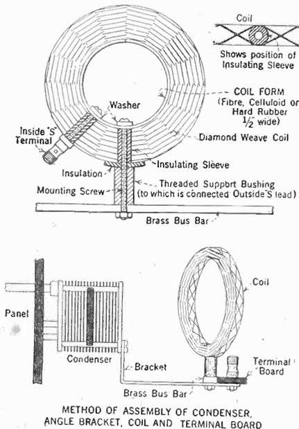
METHOD OF ASSEMBLY OF CONDENSER, ANGLE BRACKET, COIL AND TERMINAL BOARD
