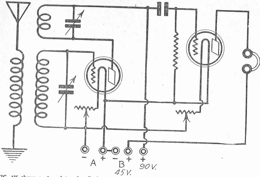
FIG. 135 shows a step of tuned radio-frequency employing regeneration in the RF stage. Wonderful results have been gotten with this 2-tube set. The primary has 10 turns, the secondary 42 turns, the fixed tickler 35 turns. The wire is No. 22 SCC. The variable condensers are .0005 mfd. There are only two controls.
