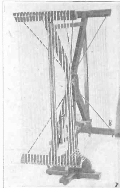
FIG. 6—Side view of loop, showing winding method.
