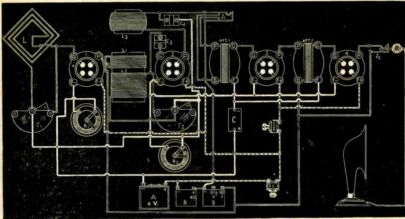
PICTURE DIAGRAM of the wiring of The Diamond of the Air, a 4-tube DX loop receiver described in the April 4, 11 and 18 issues of RADIO WORLD, with a trouble-shooting article in the April 25 issue. Note that the ground side of the secondary connects to the rotor of the variable condenser C2 and the grid goes to the stator plates, as explained in the original article and shown in the schematic diagram (April 4) but not brought out clearly in the picture diagram in that same issue.
