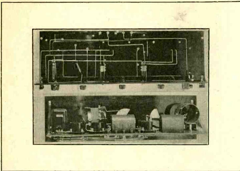
FIG. 5—Bottom view of the Twinplex circuit, showing how most of the wiring is under the subpanel. Fig. 6 (lower photo) is rear view.
