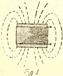
sustained. No set can be properly neutralized when such stray magnetic coupling exists. In the Neutrodyne, therefore, the coils are mounted at an angle, approximately 53.7 degrees, but varying slightly for different conditions, to minimize the stray coupling or feedback. The object is to keep oscillations, an inherent vice in tubes, under control.
