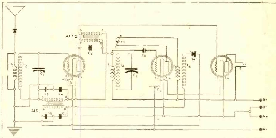
FIG. 1. Circuit wiring of the set designed to reduce static effects.
