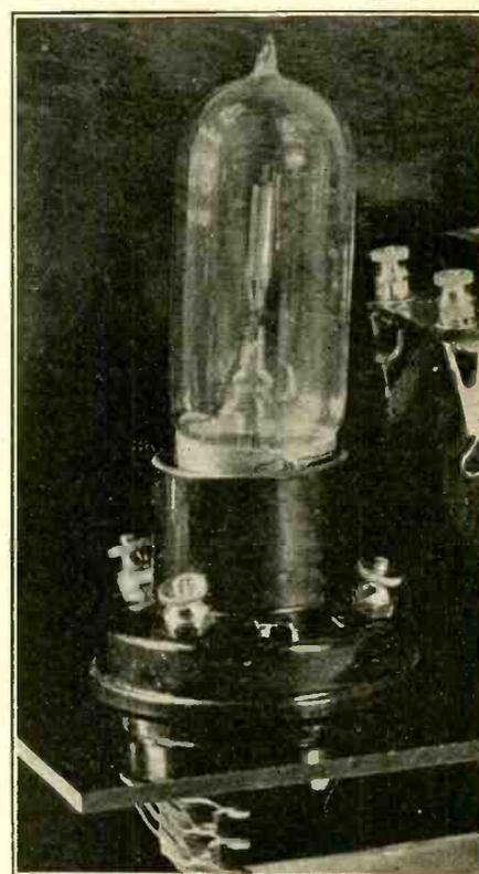
HOW a sub-panel may be mounted on top of the jacks.
