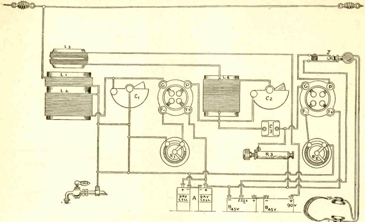
FIG. 4, picture diagram of the wiring of the Tone Beauty. This corresponds in every particular with the schematic diagram (Fig. 1).
