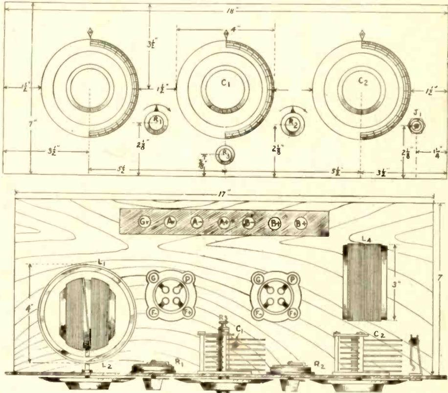
FIG. 2, the panel layout (above) and Fig. 3, the assembly plan.
