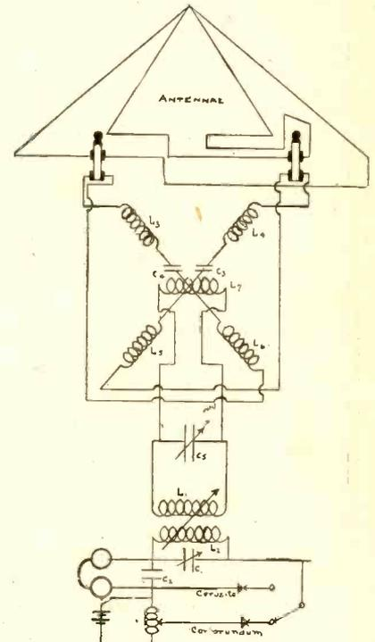
WIRING DIAGRAM of the Marconi Direction Finder. Note the switches to shut in or out the 8 ft. and 6 ft. movable antennas. A large handle controls the moving of the aerials. This finder is a very accurate instrument.
