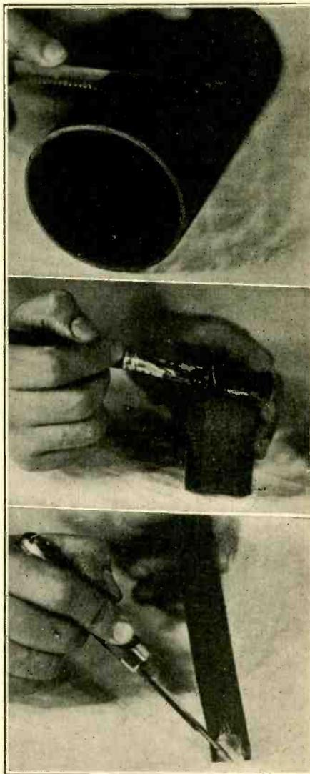
FIG. 2 (top), take a cardboard tubing, 3/8" diameter. About 1/4" from the end saw off the resulting ring. Fig. 3, clean up the ring and give it a coat of shellac. Allow to dry. Fig. 4, take a wooden stick, 10" long x 1" wide and cut two notches, one at each end. The jackknife points to the U-shaped slot at one end.
