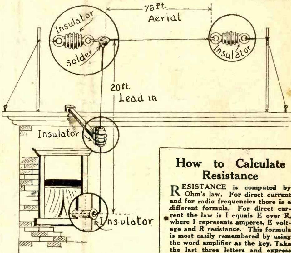
FIG. 1—The correct way for an antenna to be installed. Note where the insulators are placed, also the soldering connection.
