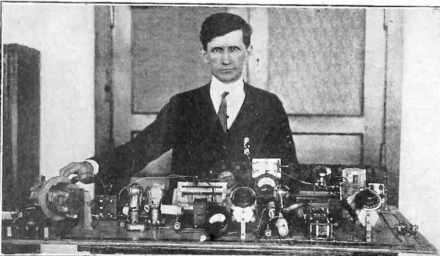
A. M. TROGNER, of the Naval Research Laboratory, operating the short-wave transmitter (40-85 meters) which he designed. This set is to be installed in about thirteen of the Naval Districts throughout the United States. (Harris & Ewing)
