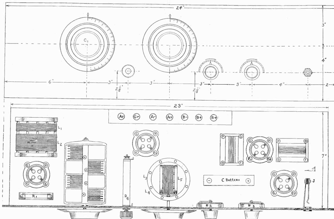
FIG. 2 (top) shows the panel layout. The switches are omitted, as their placement may be at any suitable point. The grid leak knob is between the dials. In Fig. 3, assembly plan, note that the coils are at right angles. This helps present feedback by stray magnetic coupling. R1 is the ballast resistance. R4 is the Bretwood Variable grid leak.
