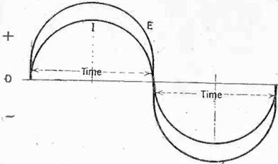
FIG. 3—A sketch showing the voltage and amperage cycle in phase.
