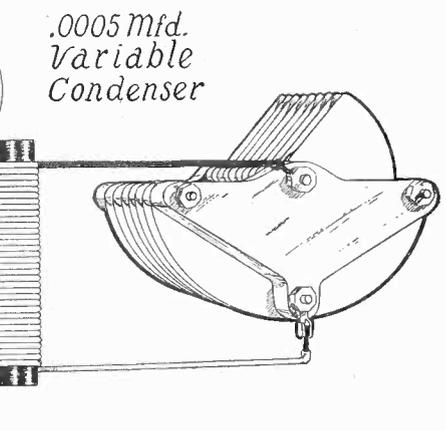
FIG. 146—A coil shunted by a variable condenser. A question mark over the coil shows that a coil which is fixed and can be tuned by a variable condenser, must have an inductance sufficient to be effective with the condenser in shunt to tune the broadcast band. For .0005 mfd. condenser use 43 turns of No. 22 SCC wire for .00035 use 56 turns; diameter of tubing 3 1/2".
