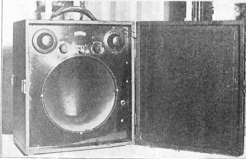
A COMPLETE 8-tube Super-Heterodyne compactly arranged in a 16x18" valise. The top picture shows the inside rear view of the receiver, the eight 199 tubes being supported on a piece of hard rubber panel. The lower photo shows the front panel, with speaker built in. The two dials control variable condensers.
