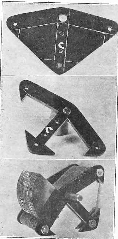
FIG 6, showing another method of cutting away dielectric end piece, preferable in remodeling condensers that lend themselves more readily to this method. Here one original mounting hole is retained and a new one drilled, the one above the C in the photo. Fig. 7 shows the insulation cut according to the pattern. The three holes for affixing the end piece to the metal plates are retained.
