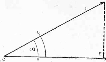
FIG. 2—A diagrammatical sketch of a lagging current. The arrows indicate the direction in which the voltage cycle and the amperage cycle go, both in opposite directions. The peculiar letter between the angle is called "alpha."
