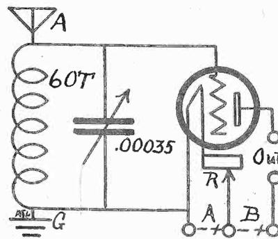
FIG. 149—A single-tube, non-regenerative receiver. This receiver is exactly the same as a crystal set, except that there is more stability and bit more volume. This is the least amount of materials that can be employed in a tube set. The tubing is 3/4" diameter.
