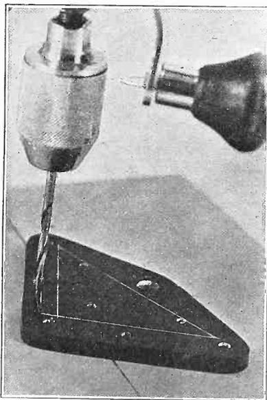
FIG. 3, two holes are drilled outside the triangle, so that mounting screws may be inserted, to enable panel mounting. Since the triangle is to be cut away, the old mounting holes will disappear.
