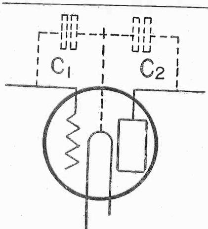
A DIAGRAM showing in symbols how capacity exists between the grid and plate elements of a vacuum tube. This is the capacity that has to be neutralized in a Neutrodyne receiver.
