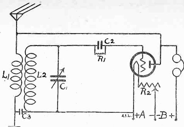
FIG. 147—A diagram of a single circuit single tube regenerative set. L1 and L2 are wound on a 3" tubing. L1 10 turns, L2 60 turns, 1/4" between two windings. This set oscillates beautifully and is a terrible interference maker. C3 is .001 mfd. C1 is .00035 (usually 17 plates).
