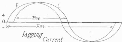
FIG. 1—Above diagram shows a lagging current, I (amperage) lagging behind E (voltage). Note the difference in time.
