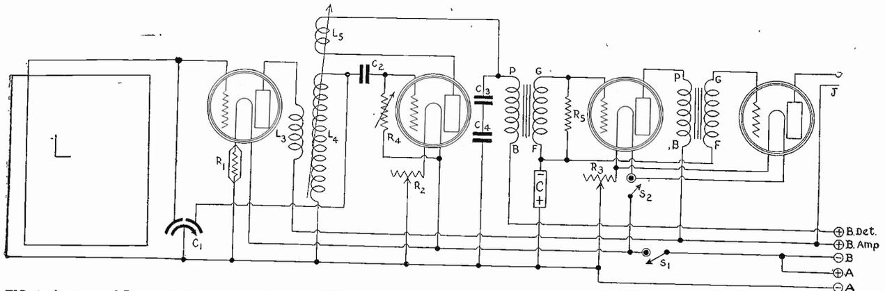
FIG. 4, the 2-control Diamond of the Air as a loop set. This is a thoroughly tested and efficient hookup and fine for Summer work, as the loop brings in less static. See next week's article for a discussion of this arrangement, particularly the matching of L4 with the loop inductance.
