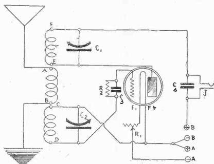
FIG. 1, circuit of the tuned plate regenerative set. The coil terminals are designated by letters, so that the novice will be sure to get the polarities right. The grid coil CD is connected in reverse fashion to the usual (incorrec) method.
