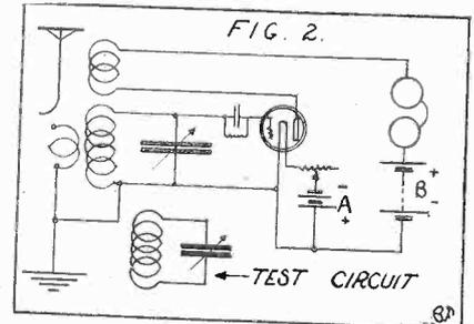
A 3-CIRCUIT single-tube receiver, with a wavemeter placed in inductive relation to the ground. How to construct all types of wavemeters will be described in the Vacation Number, June 6. There is nothing new about this set except that the antenna coil has a switch by which the aerial may be disconnected, so that you calibrate the exact wavelength that your set can receive, without the antenna (which is pure inductance) instead of making the wavelength higher than really the coil will tune to.
