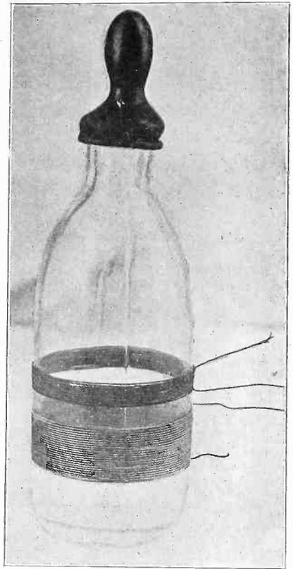
EVEN baby's bottle can be used in a radio set and to advantage. Take some No. 22 or 24 DCC wire and wind 10 turns nearer top of bottle, leave 1/2" and wind 56 turns more. Lo and behold, we now have an efficient radio-frequency transformer of the low-loss type! The coupling can be varied by simply putting the secondary nearer or further away from the primary. This is made easy by the fact that the glass is slippery and offers no resistance as does a bakelite or rubber form.
