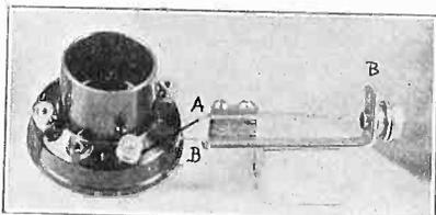
CORRECT the spring (A) of a Jack to plate, the right-angle or frame (B) to B battery.
