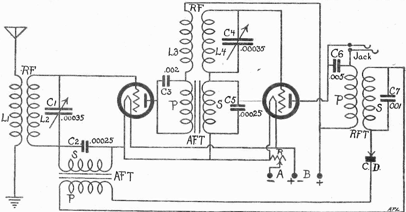
FIG. 144, a 2-tube reflex, employing an Acme radio-frequency transformer, and two General Radio or any other standard make audio frequency transformers. L1 and L2 are both wound on a 3" tubing. Use No. 22 DCC, L1, 10 turns, L2, 60. One-half inch separation between the two windings. L3 has 15 turns, L4 has 60 turns, 1/4" between two. Use No. 22 DCC. C is a fixed crystal detector. 67 1/2 volts are employed on plates of tubes. PS is a fixed RFT.
