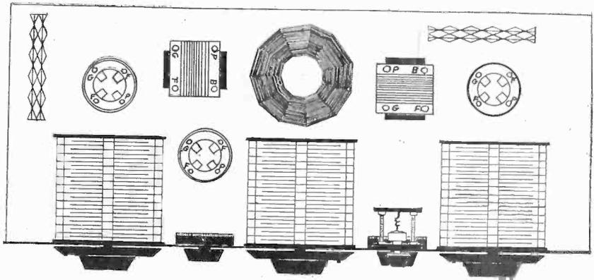
FIG. 2, the assembly plan of Wright's 3-Tube Reflex.
