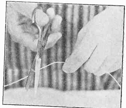
EVEN a pair of scissors comes in handy in cutting wire, although pliers are more frequently used. Scissors can easily be used to scrape off the insulation and also to cut at close quarters. (Hayden Studios)
