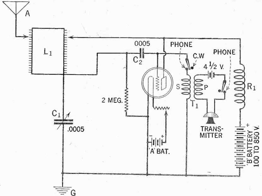
CIRCUIT DIAGRAM of the 5-watt transmitter.
