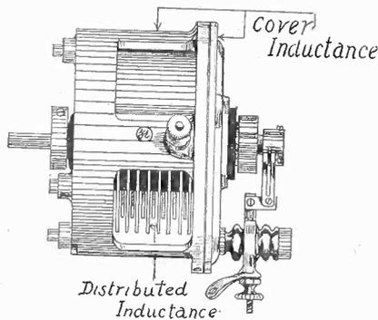
FIG. 4—Where inductance (distributed) is present in a continuously variable air condenser. Note the arrows between the plates indicating that even the material (aluminum) contains inductance.
