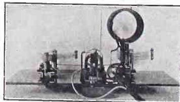
BOTTOM VIEW of the receiver, which was made without baseboard, thus necessitating a panel-mount socket.
