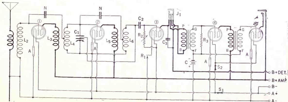
THE NEUTRODYNE, in which the neutralizing condensers are designated N. The dielectric should be air, not glass. (Fig. 5.)
