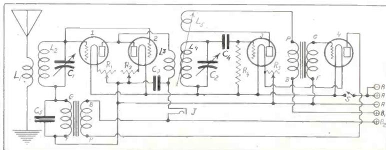
**C3, BETWEEN** the end of L3 and the A minus lead, to lower right of the second tube, is used as a bypass. C5 is also a bypass condenser in its conventional position on a reflex set, across the secondary of the first AFT (lower left). Bypass condensers should be no larger than necessary. (Fig. 3.)
