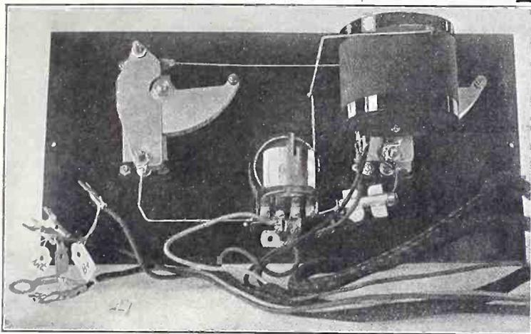
THE REAR VIEW of the set, showing the tap lead that goes to A+.
