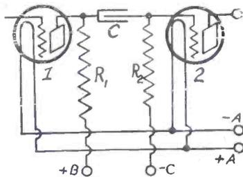
**A FIXED** condenser, C, used somewhat similarly to a grid blocking condenser. The above is a direct coupled circuit, tubes 1 and 2 being coupled by condenser, with the aid of resistors, for audio amplification. For such audio coupling C should be as large as possible. The large condensers are expensive, so .25 mfd. is a frequent compromise, yet 4.0 mfd. would be much better. The reasons are given in the text. (Fig. 2)
