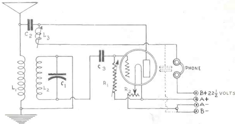
**SERIES COUPLING** by means of a fixed condenser, C2. It should be very small, say .0001 mfd., for loose coupling and large (e.g., .002 mfd.) for tight coupling. Fixed condensers used, as C2, in RF work, should have only the best dielectric. C3 is the grid condenser, used for blocking the grid current in the detector. The dotted condenser is a bypass. (Fig. 1.)
