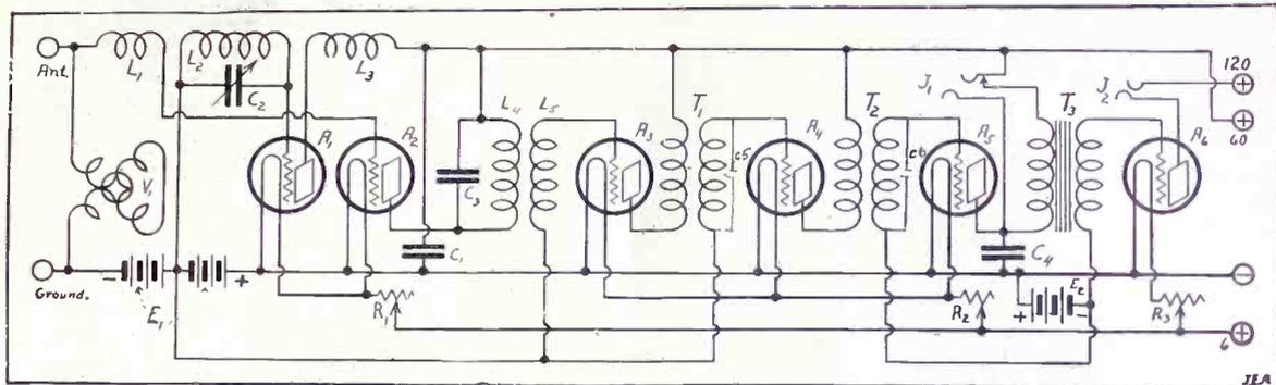
A FIXED bypass condenser across the B battery is shown above (C), to right of C4, a bypass condenser for RF currents (to right of second tube from left) should not exceed .002 mfd. The intermediate frequency condensers in the above Super-Heterodyne are C3, to right of second tube, across primary, and the ones across succeeding secondaries. (Fig. 4.)
