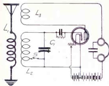
FIG. 4, a tapped secondary, with switch to short-circuit the otherwise dead end.
