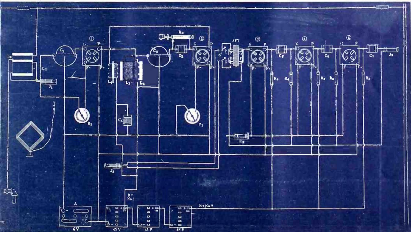
RADIO WORLD'S most popular circuit, The Diamond of the Air, shown in blueprint form. This is the 1926 model, embodying the Bernard audio amplifier. See page 5 for article on construction of this receiver.
