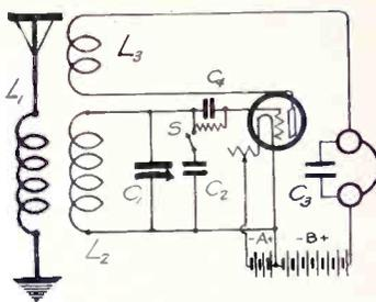
FIG. 2, a fixed condenser switched on for parallel connection with C1.
