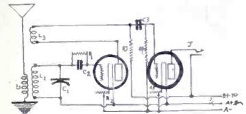
FIG. 1, the wiring diagram of the short-wave set.
