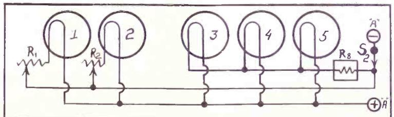
DETAIL of the filament wiring of the 1926 Model Diamond of the Air.
