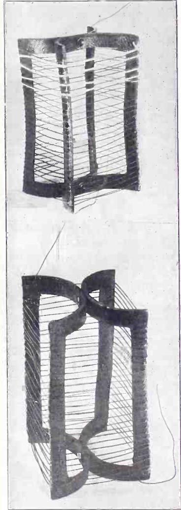
FIG. 9 (top) shows an RF transformer, 4 turns No. 18 DCC wire for primary, 25 turns No. 22 DSC wire for secondary. Fig. 10 is an impedance coil. (Hayden Photos)
