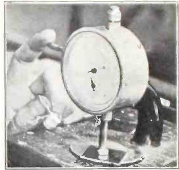
WHEN a mica fixed condenser is carefully made the thickness of the mica is measured with a meter and voltage is applied for electrical test. (International Newsreel)
