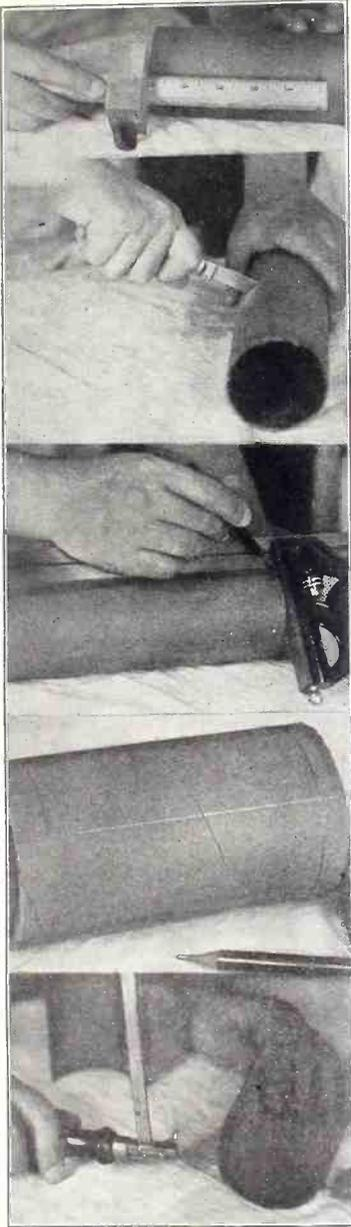
FIG. 1 (top), get a piece of cardboard tubing,  $3\frac{1}{2}$ " diameter, 6" long or so. Fig. 2 (third from top), a straight line is drawn down the tubing and another line diametrically opposite. Fig. 3. (third from top), two other lines are marked  $\frac{1}{2}$ " from the natural circumference and from the scratched one. Fig. 4 (second from top), cut the tubing at the drawn circumference 5" from the other one. Fig. 5 (bottom) shows how a scroll saw may be used rather than a knife. L.
