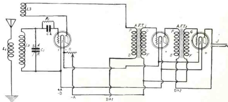
FIG. 200, showing the electrical diagram of a 3-tube set. The constants for the coil are the same as in the coil of Fig. 199. C1 is a .0005 mfd. variable condenser. C2 is the .00025 grid condenser. R1 is a 2 megohm grid leak resistance. A 6-ohm resistance is used to control the filaments of the UV201A tubes. The new UX tubes may be used here also. AFT 1 and 2 are both of the low ratio type.
