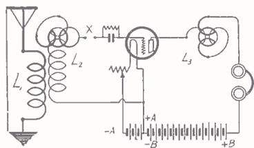
FIG. 6, a variometer used as a tuned secondary. The break at X is for a loading coil.
