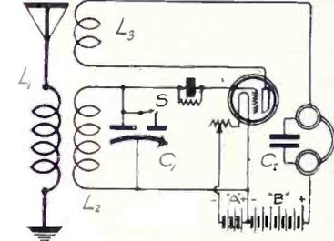
FIG. 3, how a double condenser is used, one stator being cut in by S in parallel with the other stator, or only one stator (at left) being used alone.
