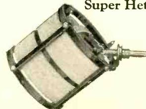
The characteristics achieved through the use of the Aero Coil principle make of this instrument the ready means to tremendously increase the efficiency of the oscillator circuit in any Super Heterodyne receiver. Pr. \$5.50
