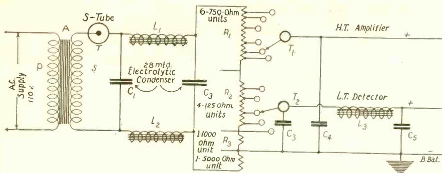
FIG. 1, showing the electrical diagram of the B battery eliminator. C3 of the 28 mfd. electrolytic condensers should be C2. R4 is the 5000-ohm unit.
