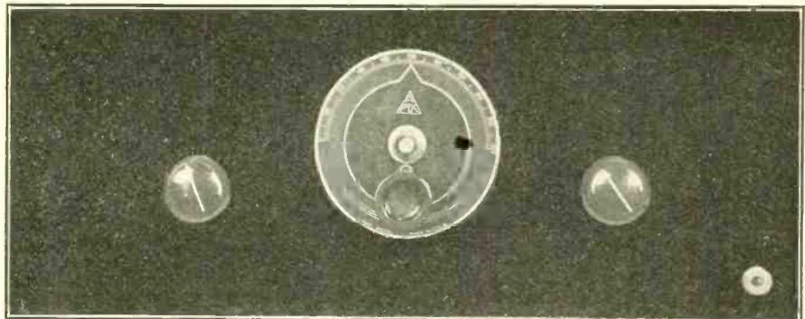
FIG. 2, the panel view of the set. The filament control jack is at right (Kadel & Herbert)
