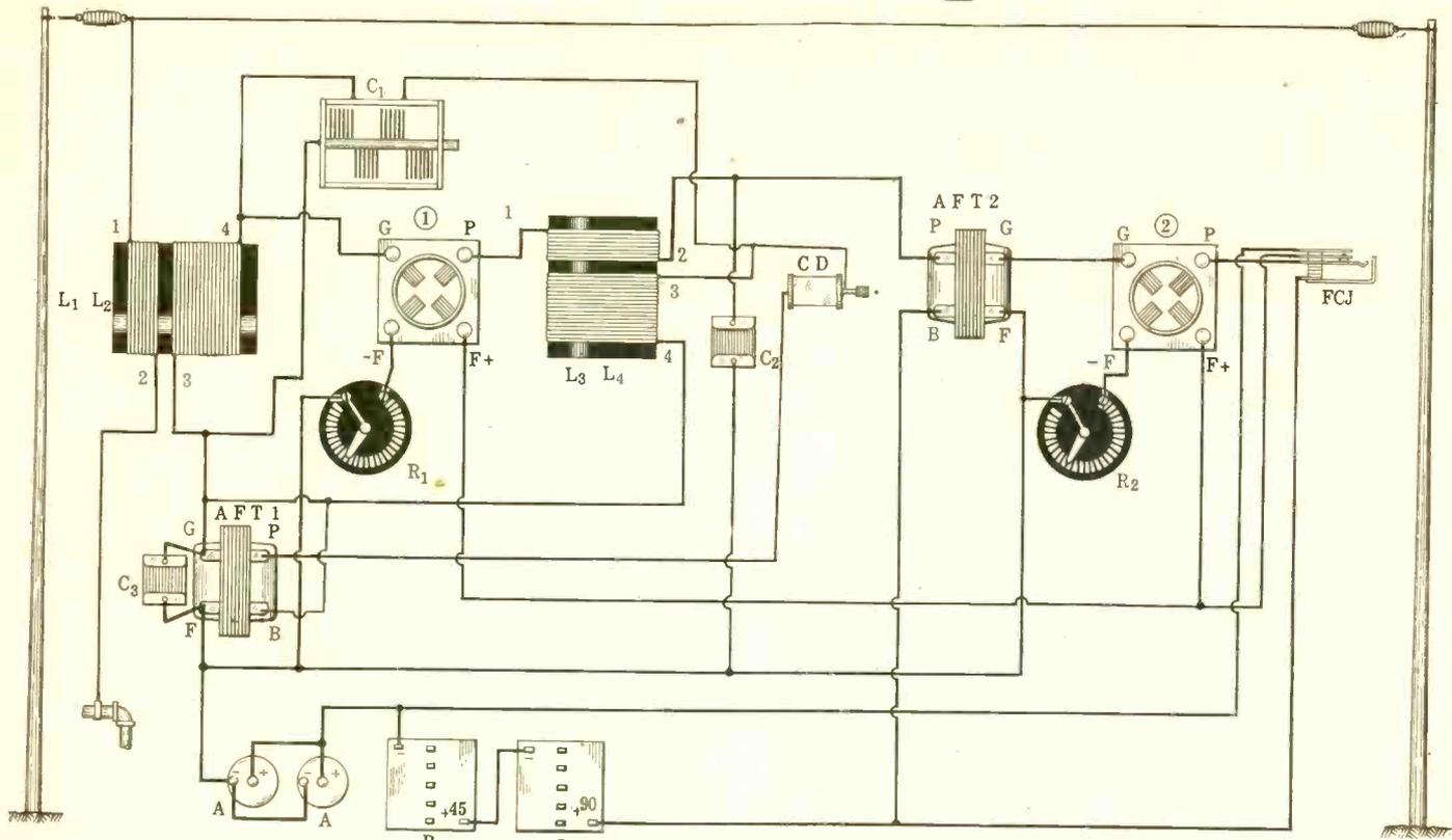
FIG. 1, a picture diagram of the wiring of the 2-tube speaker reflex that uses only one dial for tuning. The coils are marked for polarities that correspond with the explanation in the text.
