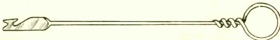
ALL sewing can be done with this needle before removing a basket-weave coil from the pins.
