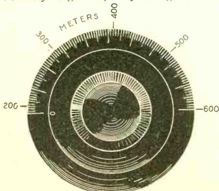
FIG. 3, how the stations are separated on the "Straight-Line Wavelength Condenser."
