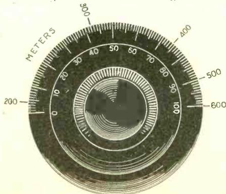
FIG. 4, showing the great separation on the lower end of the dial on a "Straight-Line Frequency Condenser." Note the crowding at the higher wavelength part of the dial.
