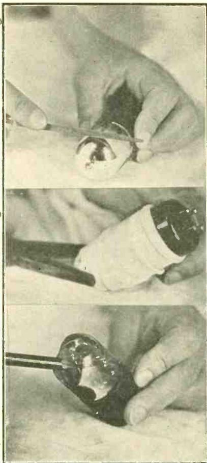
FIG. 1 (top), a circle is filed around a burnt-out tube, near the top. A piece of cloth is then wrapped around (Fig. 2). Then hit the glass with a pair of pliers. (Fig. 3). The wrapper is then removed. If the break is jagged you can make a smooth circle by breaking off the glass with pliers at the circle.
