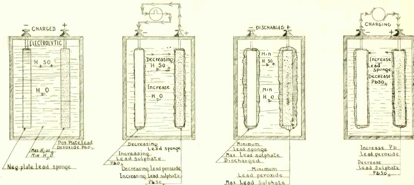
FIG. 200, showing the action which goes on inside of the storage battery. Note that in the first diagram the electrolyte is called electrolytic. This is not correct.
