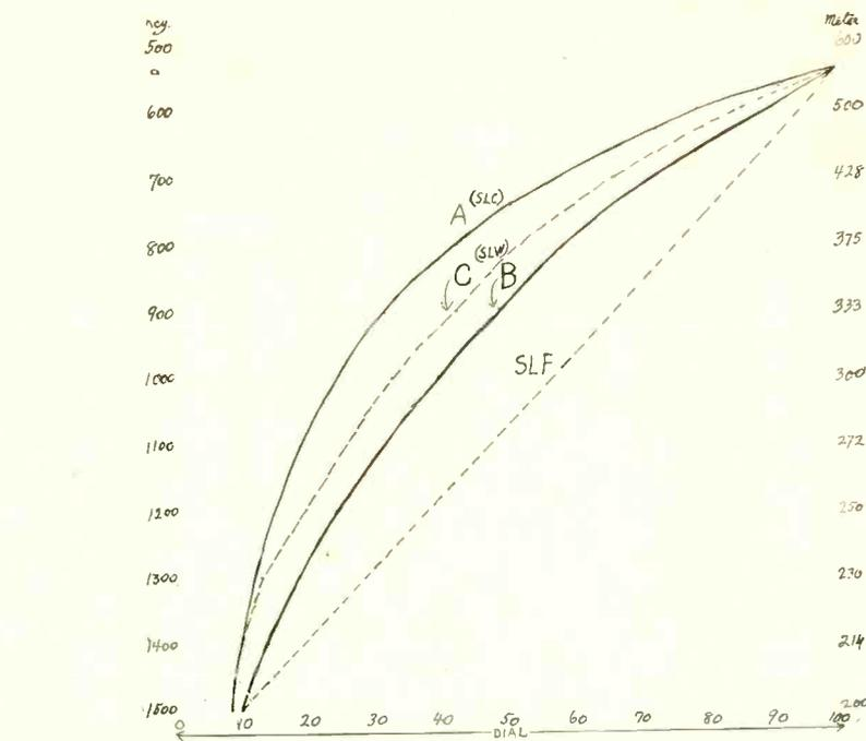
FIG. 2, a comparison of the curves of all the four specimens, (1), the SLC condenser, ordinary dial, "A"; (2), SLW condenser, ordinary dial, "C"; (3), SLC condenser, frequency type dial, "B"; and (4), a SLF condenser curve, ordinary dial. The above is a frequency chart (numbers at left are kilocycles), while Fig. 1 is a wavelength chart.
