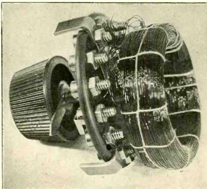
FIG. 12, the coil mounted on the back of the switch and the taps fastened to switchpoints.
