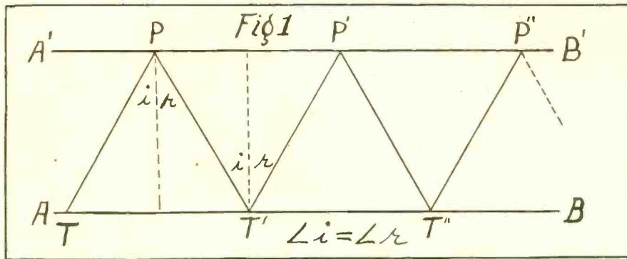
FIG. 1, representation of the action presumed when the Heaviside layer theory is applied.
