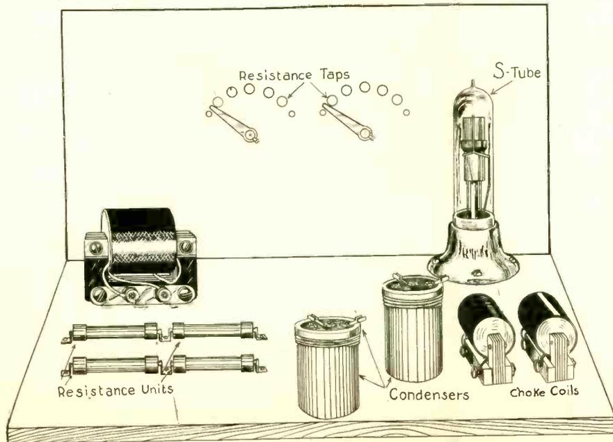
FIG. 4, showing the picture diagram of how the eliminator parts should be placed. Note that there are only 2 choke coils seen. The third one is hidden behind the others.
