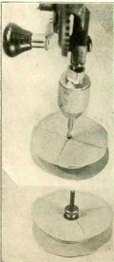
FIG. 5, center the larger circle and make a hole with a No. 27 drill. Next (Fig. 6) put a  $\frac{6}{32}$ " screw in the hole and fasten tight.
