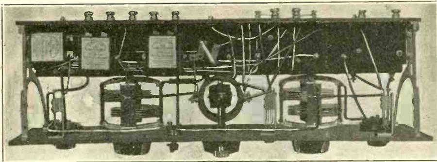
FIG. 5, the bottom view of The Diamond, showing how much of the wiring is done under the socket shelf, which is supported by brackets. The three .25 mfd. fixed condensers needed for the Bernard audio hookup are shown at left. The loop jack is at right in this photo.
