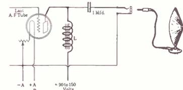
HOW the final audio output may be connected from plate to filament. L is a choke coil.
