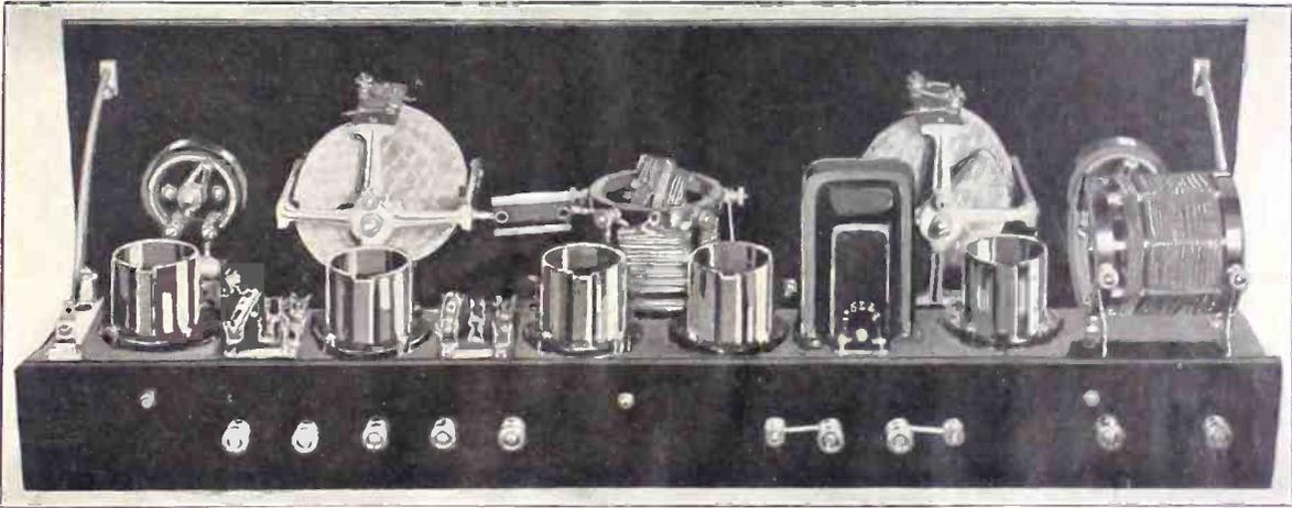
FIG. 7, rear view of the 1926 Model Diamond of the Air. The binding posts, right to left on the supporting strip, are (1) aerial; (2) ground; (3) detector plate; (4) P post of AFT; (5) B post of AFT; (6) B+ No. 1; (7) A minus; (8) A plus; (9) B minus; (10) B+ No. 1, and (11) B+ No. 2. Note (6) and (10) are the same lead. The two are interconnected behind the supporting strip that holds the binding posts, as (10) better accommodates the battery cable lead. Posts (4) and (5) are T and T in Fig. 8.
