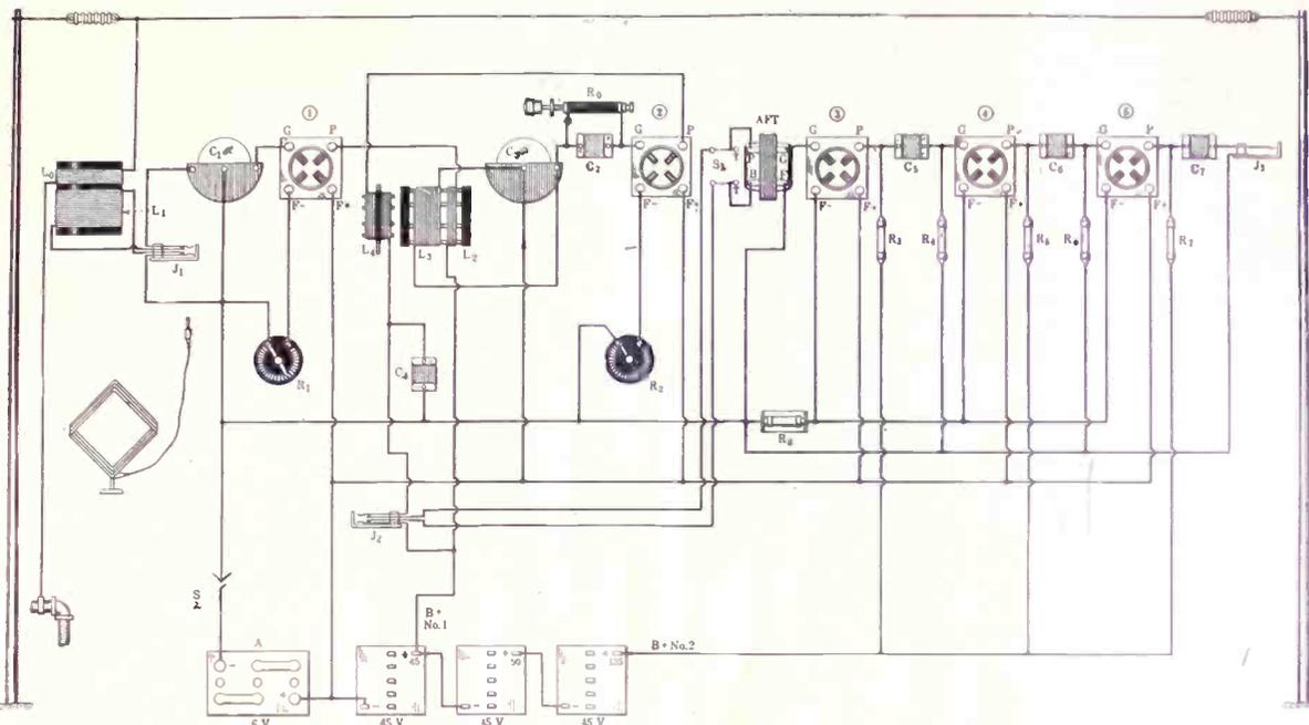
FIG. 8, the circuit diagram of the 1926 Diamond shown in picture form, with the A battery switch S2 used as a master switch, to turn the set on or off as a unit.
