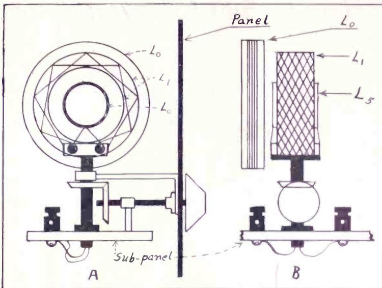
FIG. 2, the side and back views (A and B) of the coil as mounted.
