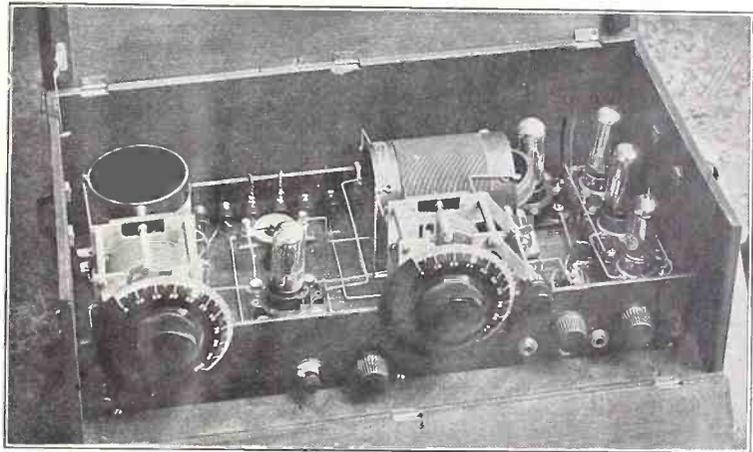
A VIEW of the assembly of the portable set.
