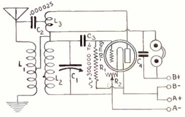
FIG. 1 showing the electrical wiring diagram of the receiver, described in the text.
