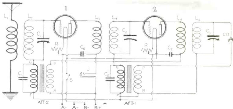
FIG. 202, a 2-tube Inverse Duplex. L1, the primary, has 10 turns wound on a 3 1/2" tubing 4" high, with No. 24 DSC wire. There is 1/4" space left and L2, the secondary, has 43 turns. L3 and L5 are the same as L1. L4 and L6 are the same as L2. C1, C2 and C3 are variable condensers having a capacity of .0005 mfd. C6 and C7 are .001 mfd. condensers. C4 and C5 are both .0001 mfd. condensers. The rheostats R have a resistance of 20 ohms. CD is the crystal detector.
