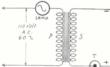
FIG. 3, showing how to hookup the "S" tube for charging purposes. T is the S tube.
