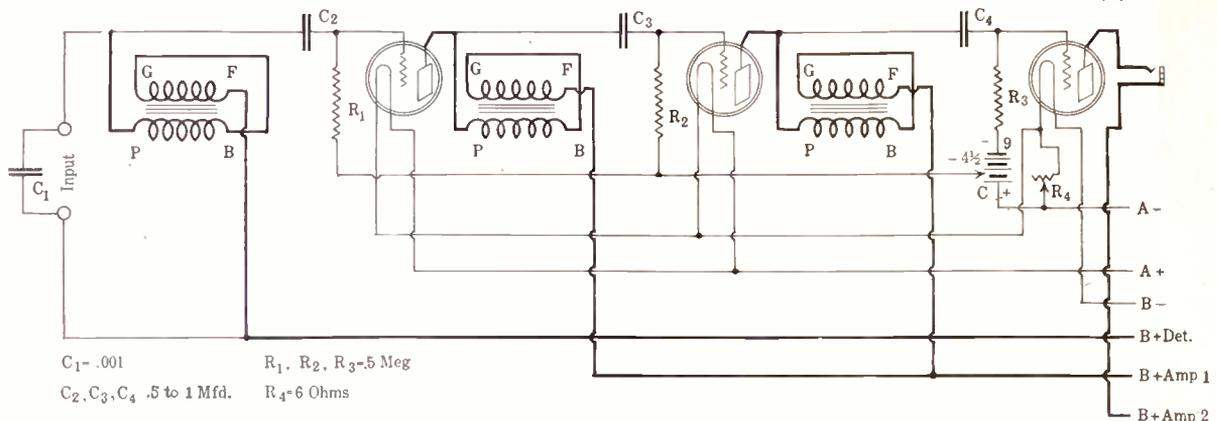
THREE stages of impedance-coupled AF amplification. Transformers are used as the choke coils, the primary and secondary of each being connected series-aiding. The markings are not correct for all types of transformers.
