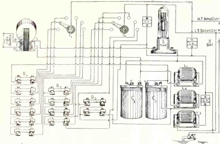
FIG. 1, showing the picture diagram of the tube B battery eliminator. Note that the last two resistances of the 4-125 ohm batch.
