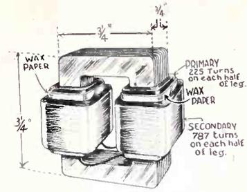
FIG. 2, showing how the AC transformer should be wound. Note the waxed paper separating the primary and the secondary windings. There is also waxed paper underneath the primary windings.
