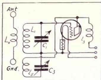
FIG. 1, the wiring diagram of the circuit that uses the secondary as a loop.
