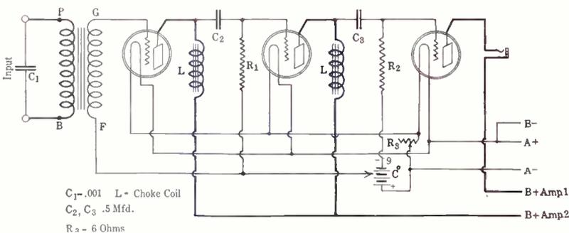
ONE transformer stage and two impedance steps. The choke coils L may be audio-transformers as in the hookup for three impedance-coupled stages. For  $C_2$  and  $C_3$  one may use .006 mfd., but .5 mfd. or even 1.0 mfd. would be better.
