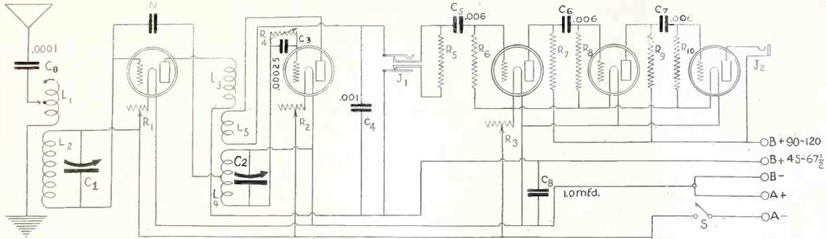
FIG. 1, wiring diagram of the 5-tube Browning-Drake receiver, including 3-stage resistance-coupled audio-amplifier.
