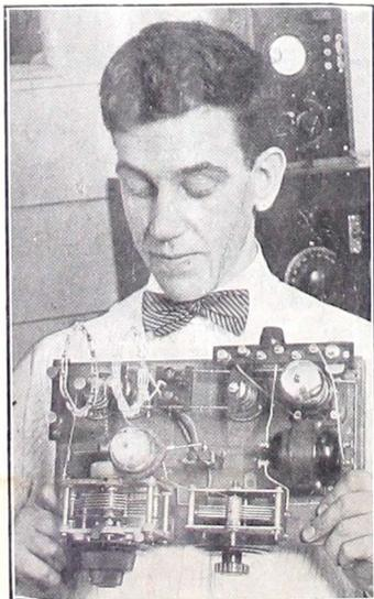
HERE IS the amateur's delight, a short wave low-loss receiver. The circuit is the standard regenerative type, with a tickler employed in the plate circuit and will tune from 20 to 110 meters. The base of the tube was taken off so that there would be no extra capacity to raise the wavelength of the set or make it hard to control. The coils are of the air wound type. Note the large porcelain insulators on the baseboard.
