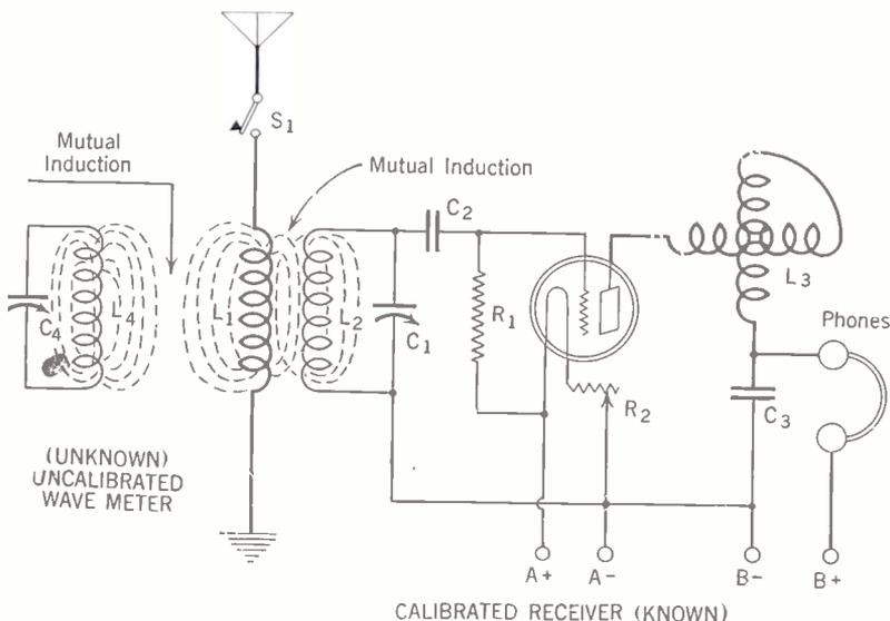
IF you know the dial readings of your regenerative receiver you may calibrate a wavemeter. C4 is a .0005 mfd. variable condenser. L4 is a 50-turn coil, wound on a tubing 3" in diameter with No. 22 DCC wire.
