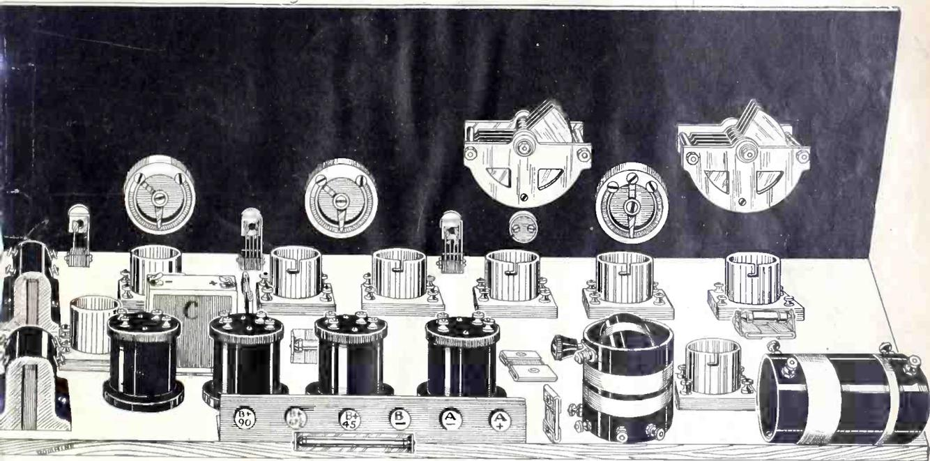
REAR VIEW of the 8-Tube Standard Super-Heterodyne showing the placement of the parts. See article on page 8.
