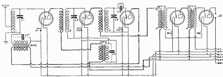
CIRCUIT network of a reflexed receiver. Det. plate lead is continuous.
