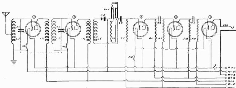
A TUNED radio frequency set with crystal detector.
