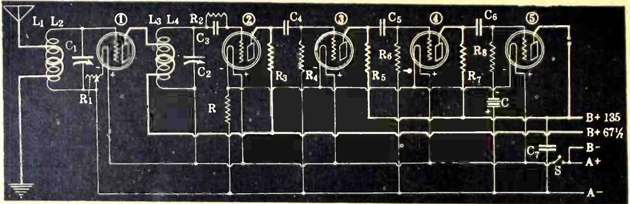
THE ELECTRICAL diagram of the 2-C, 5-tube receiver, described in the January 2 issue of RADIO WORLD by Capt. P. V. O'Rourke. L1 and L3, the primaries shown by the heavy white lines, are wound in the middle of the secondary and side by side with the continuation of the secondary winding. The secondary, using .00035 mfd. variable condensers, consists of 65 turns on 3" diameter.
