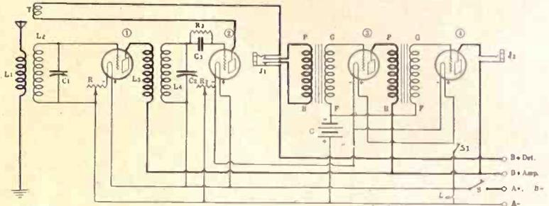
FIG. 1. THE TICKLER COIL is used in both the radio frequency and detector stages by the method shown in the diagram. The method is a departure from the conventional in hookups, and is suggested by the author as a means of remedying critical tickler adjustment.
