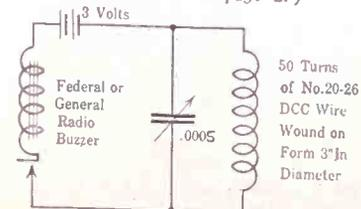
FIG. 6—Buzzer-driven coil and condenser which make ideal home-made wave meter for testing this set.
