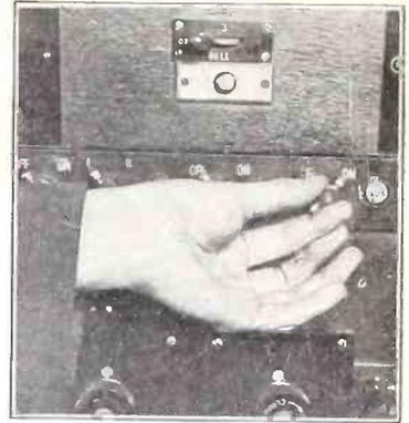
WITH the automatic SOS flash switch shown above, the operator at a broadcasting station can instantly notice if a distress signal is in the air and notify the announcer. This switch is used by WEAf. The system is much better than the old one, where the operator had to sit with the phones on his head to catch this signal.
