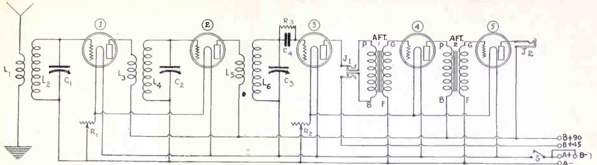
FIG. 256 showing the 5-tube TRF receiver.
