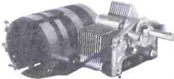
The heart of the SUPERADIO Type G Antenna Coupler showing the special coil and efficient S. L. W. Condenser.
