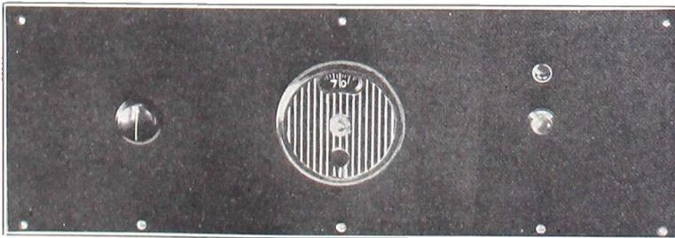
THE PANEL view of the 5-tube receiver diagrammed on the opposite page. The knob at left is the RF rheostat, R1 in Fig. 1. The switch at right lights or unlights all five tubes. The aperture above it is an opaque maroon window, illuminated by a pilot light when the set is "on." In center is the single tuning control, a dial that makes any condenser that is not straight-line frequency tune just as if the condenser were such. (Fig. 3.)
