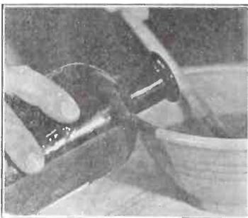
IN making a storage battery solution, always add the acid (sulphuric, H<sub>2</sub>SO<sub>4</sub>), slowly to the water, and not the water to the acid. If the opposite method is employed, a boiling and sputtering of the solution will take place. After each few drops of the acid are added in the correct fashion, stir carefully.
