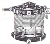
"Bruno" short wave tuner wound on quartzite meters with .00025 sens. ribbon wire...\$5.00
