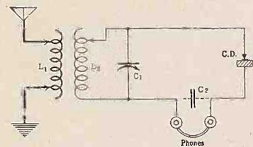
THE SCHEMATIC diagram of a simple and effective crystal receiver, wherein are used a tapped radio frequency coil, which should have a variable primary; a variable condenser, having the proper capacity to shunt the secondary; a crystal detector; a .001 mfd. fixed condenser and a pair of phones.
