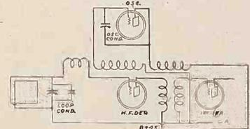
THE ELECTRICAL diagram of the frequency changing system, or the oscillator and modulator (first detector) used in Western Electric Super-Heterodynes. The Hartley oscillator is employed.
