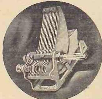
The most important feature of this new condenser is the elimination of all insulating material between the frame and the stator plates. This is accomplished by using as a shaft a rod of new insulating material.
