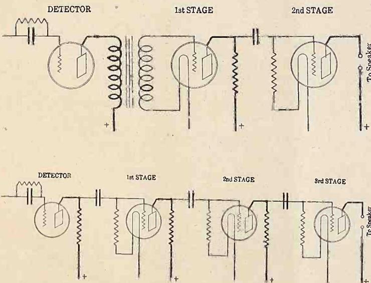
THE CIRCUIT diagrams of two popular forms of AF amplifiers. At the bottom is shown a 3-stage straight resistance coupled AF amplifier, while on top is a diagram of a stage of transformer coupled and a stage of resistance coupled AF amplification.
