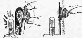
The Bruno Ruby Light Switch is a combination A battery switch and pilot light. When the knob is turned to the right, the bulb lights up, the set is on. When the knob is pressed, the set is turned off. Single hole panel mount. Price, less bulb..... **75c**
