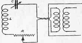
FIG. 4 The phantom antenna used in the tests.
