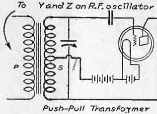
FIG. 6 A circuit better adapted for measuring low audio frequencies.
