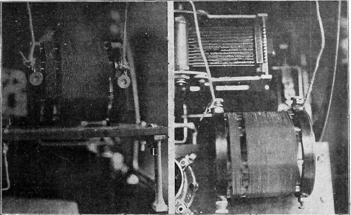
HOW to measure to capacity of your antenna-ground system. The coil at left has untuned primary connected to aerial and ground. The dial setting is noted. Then these leads are connected instead to the grid and grid return and the new dial setting noted. The difference discloses the approximate capacity of the antenna-ground system. See article on and other photographs on page 5.
