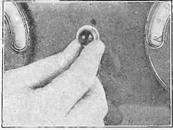
A RUBY LIGHT SWITCH is an ornament to any set. Turn the ruby to turn on the set, and a red light glows. Press the ruby and the light goes out, turning off the tubes.
