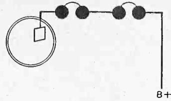
**IF TWO** or more pairs of phones or speakers are connected to a set they should be in series (as above), and not in parallel. Otherwise volume declines considerably.
