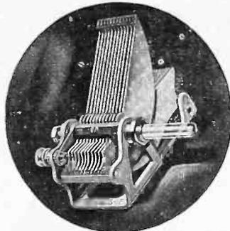
The most important feature of this new condenser is the elimination of all insulating material between the frame and the stator plates. This is accomplished by using as a shaft a rod of new insulating material. The shaft is the only insulation used in the condenser, therefore body capacity is reduced to a minimum.
