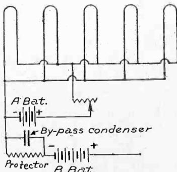
HOW to connect a device to protect tubes from blowout. Arrow indicates by-pass of protector.
