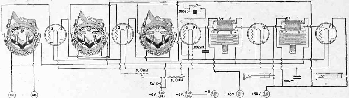
THE CIRCUIT DIAGRAM of the wiring of the receiver.
