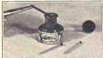
A PIECE OF PAPER, dipped in India ink, makes a grid leak of unknown resistance and short life, but handy in an emergency.
