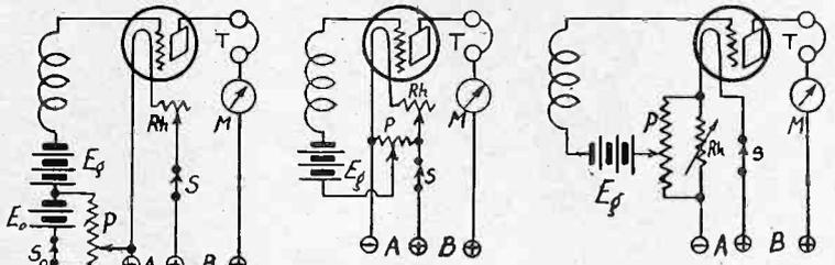
FIGS. 2, 3 AND 4, left to right, show grid bias control where a biasing battery and potentiometer are used.
