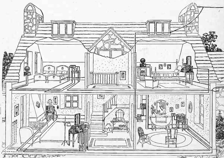
ISOMETRIC view of the model radio house described on this page, showing position of radio receivers and loud speakers. Note outlets in baseboards, remote control switches and battery compartment on second floor. Speaker in the living room may be plugged in porch circuit. The antenna and other wiring, while shown exposed, is inclosed in walls.
