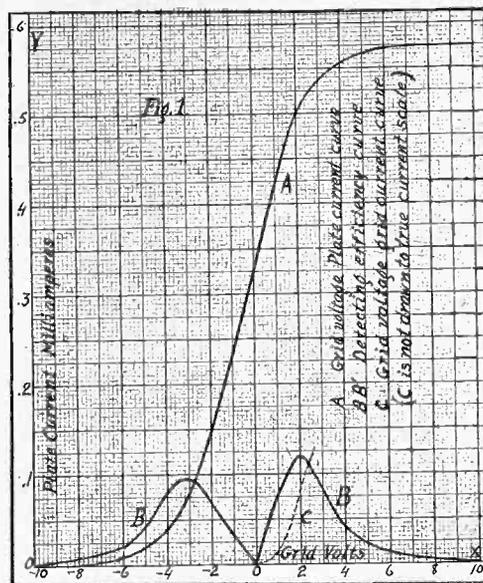
THE grid voltage, plate current curve of a vacuum tube.
