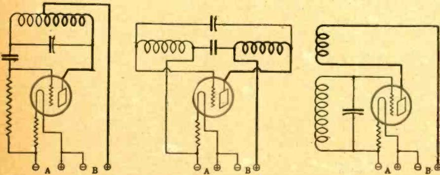
THREE POPULAR oscillator systems, employed in Super-Heterodyne. The most stable of the three is the 3-circuit tuner, shown at the right.
