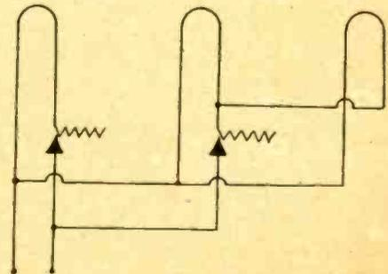
THE ABOVE electrical diagram shows how to connect up one rheostat to control the filament of the detector tube and another rheostat in a 2-stage audio amplifier circuit, for filament control.
