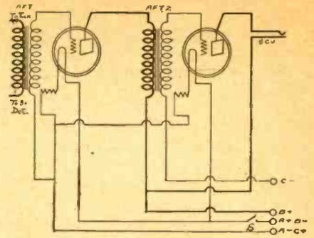
THE SCHEMATIC diagram of a 2-stage transformer coupled AF amplifier, with the proper connections for the installation of a power tube. The "To Tick" connection may go to the tickler post in detector plate circuit or to only the plate post of detector tube. Ballast resistors control the filaments of both AF tubes. Note the C battery connection.
