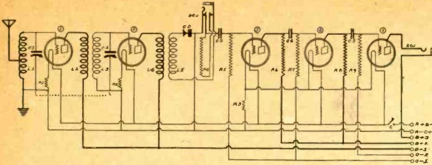
A 5-TUBE quality receiver, employing two stages of tuned radio frequency amplification, a crystal as a detector and three stages of resistance coupled audio frequency amplification. An untuned RFT is used to couple the RF output to the detector input. Ballast resistors are used throughout for filament control.
