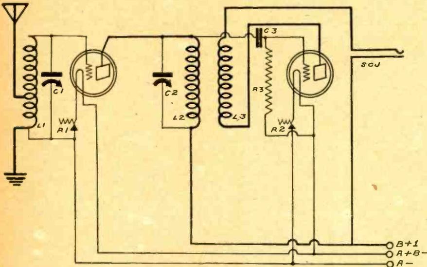
THE ELECTRICAL diagram of a 2-tube receiver, employing a regenerative RF and detector tube. This set is quite critical, but will give excellent results when properly controlled. Impedance coupling is used.
