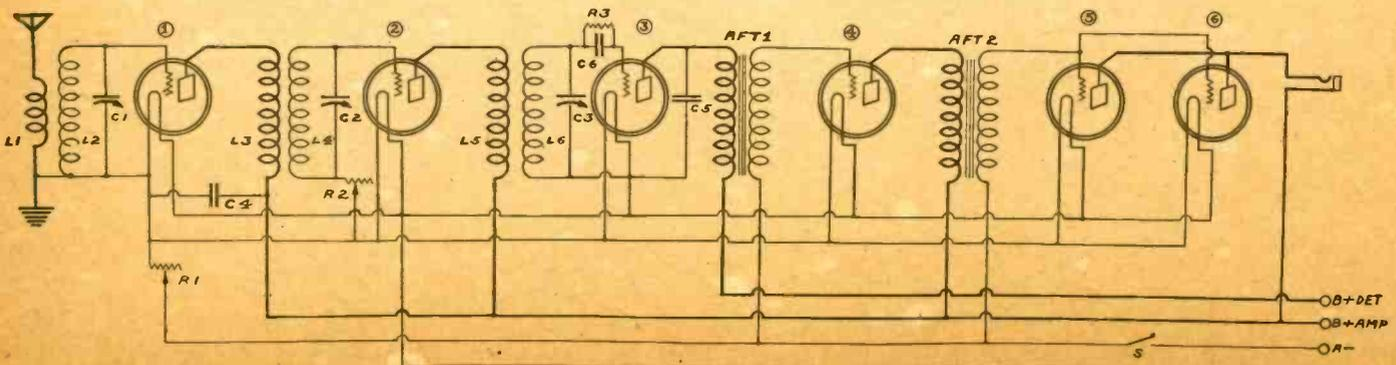
A 6-TUBE TRF receiver. Transformer AF coupling is used. Two tubes are used in the last AF stage, so that the output is balanced and free of distortion. A single rheostat is used to control the filaments of all the tubes.
