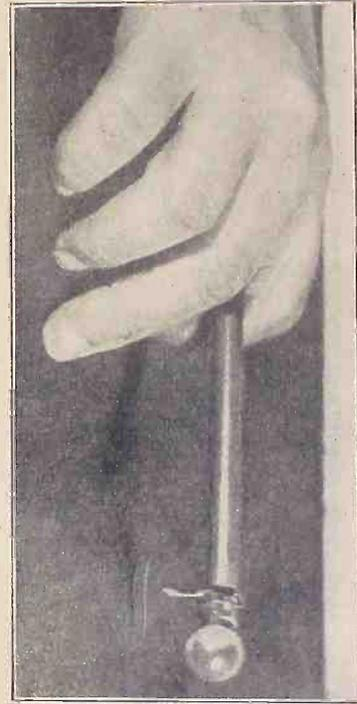
A SMALL 3-volt lamp mounted on a stick suitably connected to dry cells gives a handy light when working in a set on trouble shooting.
