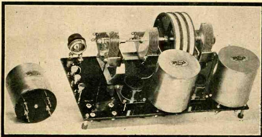
**A VIEW of the Welty RF unit, showing the interchangeable RF coils and the localized control tuning. Note the rugged construction of the sub-base. A coil with the four terminals at the base is shown to the left.**
