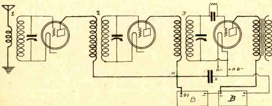
WHERE to connect the by-pass condenser in the radio frequency side of a TRF set is diagrammed above, at point X. M indicates the common B voltage terminal for the RF amplifier tubes.
