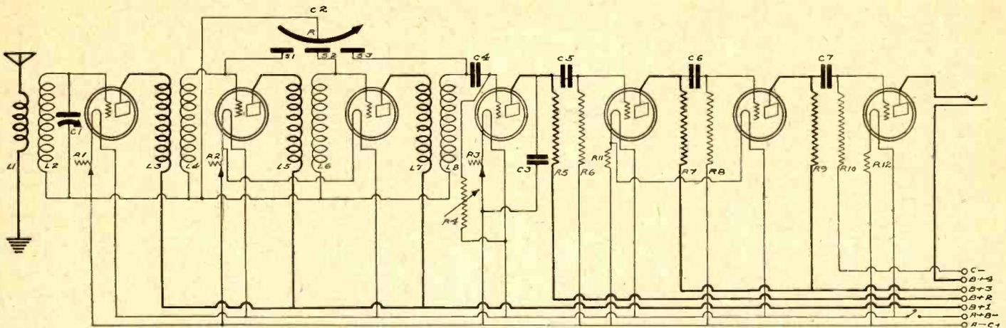
A 7-TUBE receiver, wherein three stages of tuned radio frequency amplification, a non-regenerative detector and three stages of resistance coupled audio frequency amplification are employed. A single condenser is used to tune the secondary of the first or antenna RFT, while the secondaries of the other RF's are tuned by a triple condenser. Standard RFT can be used. The grid return of the detector tube is made to plus A, through the variable grid leak.
