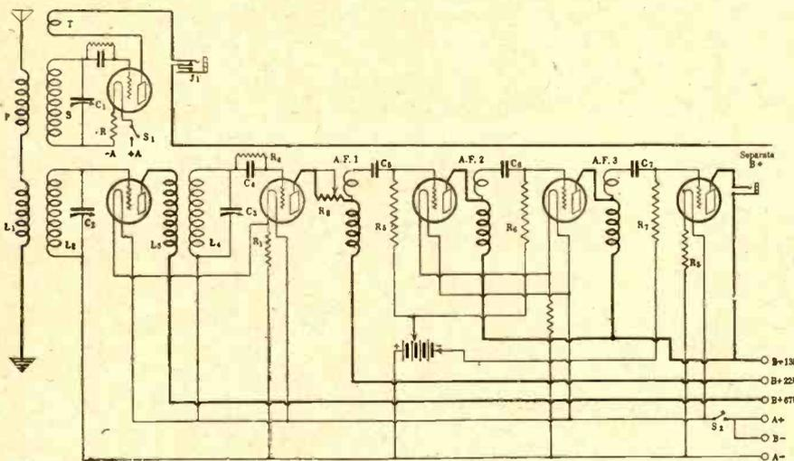
A COMBINATION 1 and 5-tube receiver. The 1-tube receiver may be used for two purposes, as a wavetrapp and as an individual receiver. The detectors in both sets are regenerative.
