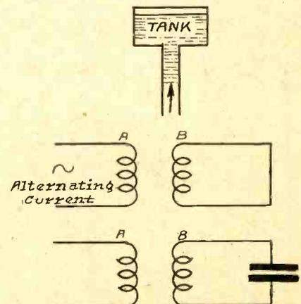
IF DC is applied to condenser plates, the charge is held intact, until saturation point; with AC the charge alternates. Using the tank as an analogy, with DC, the water stores up; with AC, it fills and empties, etc.
