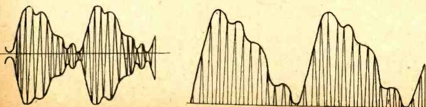
HOW THE resultant modulated carrier wave appears before and after rectification.
