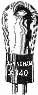
the tube works well even on only 4½ volts. The effected voltage applied to the plate should not exceed 180 volts with suitable bias. With a .25 meg. plate resistor this means the voltage source may be 300.
