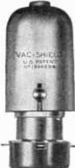
THE invention of these non-magnetic shields for Type 201-A or the new Type 222 Tubes prevents inter-stage coupling and electro-static effects, overcoming stray capacities that make tuning of distant stations so difficult.
