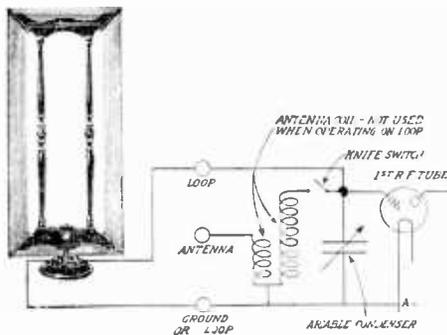
HOW the antenna coil is disconnected in a tuned RF set and a Bodine loop connected in its place is shown at left. A knife switch may be used so that the antenna coil may be cut in at will, but the loop should then be disconnected. At right is a method of using a midtap loop with Neutrodynes particularly. This method affords greater stability but lesser volume.
