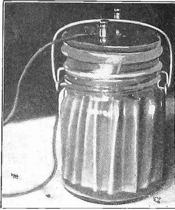
THIS depicts an electrolytic condenser built according to the description given in the accompanying article. It has a capacity of over 3,000 mfd., having been formed at about 7.5 volts. Used as a ripple remover it is quite effective.
