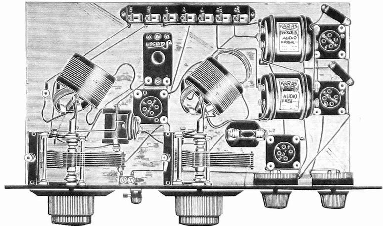
POINT-TO-POINT WIRING is used. This keeps leads short and efficiency high. The rheostats at right control volume and sensitivity.
