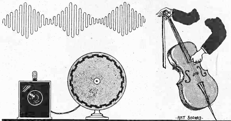
**THAT THE HARMONICS OF A PLUCKED CELLO STRING ARE NOT EXACT MULTIPLES OF THE FUNDAMENTAL CAN BE PROVED WITH THE AID OF A VACUUM TUBE OSCILLATOR. TUNE OSCILLATOR TO EXACT UNISON WITH THE FUNDAMENTAL OF PLUCKED STRING. THEN COMPARE THE HARMONICS OF THE OSCILLATOR WITH THE HARMONICS OF THE STRING. BEATS WILL BE HEARD. TO AVOID CONFUSION IT MAY BE NECESSARY TO SUPPRESS THE FUNDAMENTAL OF THE OSCILLATOR TO MAKE THE COMPARISON.**
