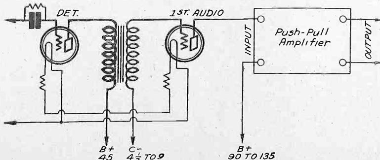
HOW THE OUTPUT OF A STAGE OF TRANSFORMER COUPLED AUDIO FREQUENCY AMPLIFICATION IS HOOKED ON TO THE INPUT OF THE GENERAL RADIO TYPE 441 PUSH-PULL AMPLIFIER IS DIAGRAMMED ABOVE.
