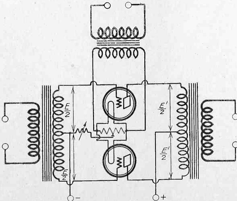
ONE STAGE OF PUSH-PULL AMPLIFICATION WITH AC HEATED FILAMENTS. THE INPUT VOLTAGE  $E$  IS DIVIDED EQUALLY BETWEEN THE TWO TUBES. EACH AMPLIFIED HALF  $E/2$  APPEARS ACROSS HALF OF THE PRIMARY OF THE OUTPUT TRANSFORMER, AND THE TOTAL OUTPUT VOLTAGE IS  $E'$ .  $R$  SUPPLIES THE GRID BIAS WITHOUT DETRIMENTAL EFFECTS.
