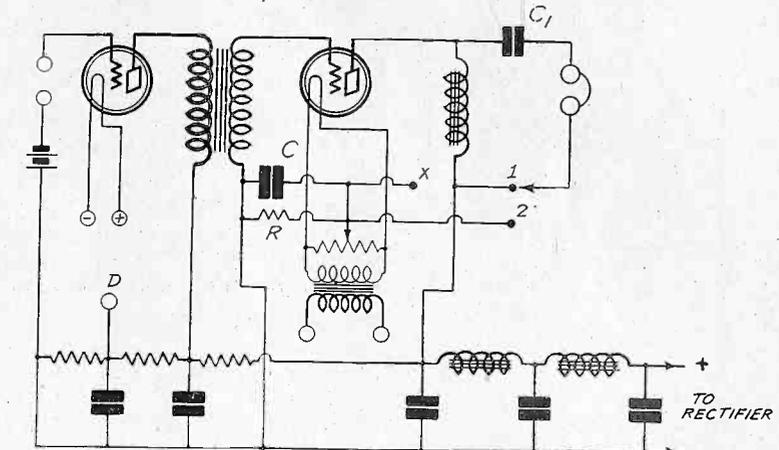
THIS DIAGRAM ILLUSTRATES THE EFFECTS OF THE GRID BIAS RESISTOR ON THE QUALITY OF REPRODUCTION, AND IT INDICATES THE PREFERRED CONNECTIONS OF BY-PASS CONDENSERS AND THE LOUD-SPEAKER TO MINIMIZE THE EFFECTS.
