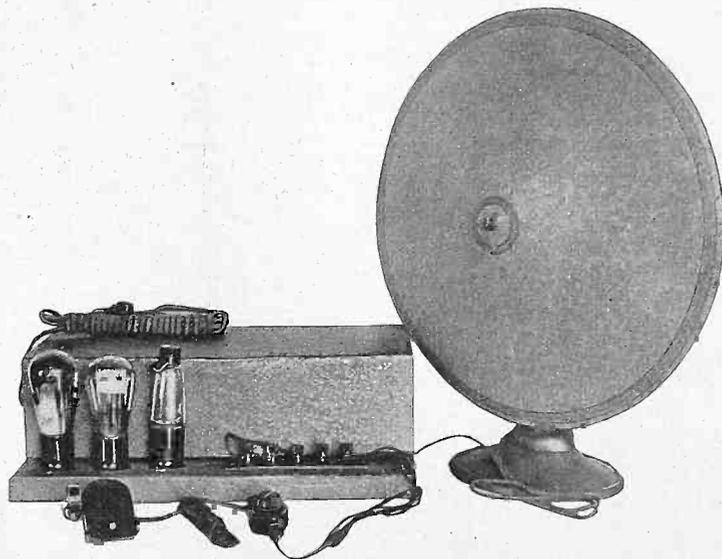
A POWER AMPLIFIER AND B SUPPLY, WITH PHONOGRAPH PICKUP [PHONOVOX] INTRODUCED IN A SPECIAL WAY, HAS BEEN DEVELOPED BY LOUIS G. PACENT. AN ADVANCE VIEW OF THE EXTERIOR IS SHOWN. SOON THE CONSTRUCTION WILL BE DESCRIBED. THE TUBES USED ARE ONE 281 (RECTIFIER) ONE 227 OR KELLOGG OR McCULLOUGH, AND ONE 210. IT IS ESPECIALLY ADAPTABLE FOR HOUSING IN PHONOGRAPHS.
