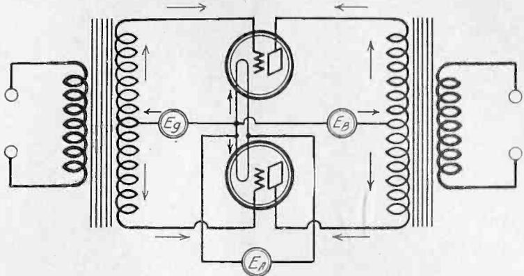
A PUSH-PULL CIRCUIT ILLUSTRATING HOW DISTURBANCES IN THE POWER SUPPLY ARE BALANCED OUT. THE ARROWS INDICATE THE DIRECTION OF THE CHANGES IN THE CURRENTS OR THE POTENTIALS DUE TO A DISTURBANCE. NOTE THAT THE CURRENT ARROWS IN THE TWO HALVES OF THE PRIMARY OF THE OUTPUT TRANSFORMER ARE IN OPPOSITE DIRECTIONS. HENCE THE DISTURBANCE DOES NOT APPEAR IN THE SECONDARY. IT MAKES NO DIFFERENCE WHETHER THE DISTURBANCE APPEARS IN EG, IN EB OR IN EA.
