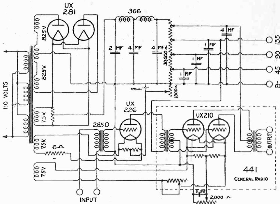
COMPLETE CIRCUIT DIAGRAM OF THE PUSH-PULL AMPLIFIER AND POWER SUPPLY DESCRIBED BY MR. WILSON. AN OUTPUT VOLTAGE OF 750 VOLTS DC IS PROVIDED FOR.
