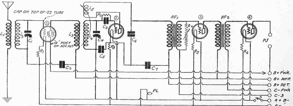
THE FOUR TUBE MODEL. WHEN THE FIFTH TUBE IS ADDED IT IS PLACED ELECTRICALLY JUST AHEAD OF THE DETECTOR. THE VOLUME CONTROL CLAROSTAT IS PUT IN THE B+ AMP. LEAD AT THE ANGLE OF THAT LINE JUST BELOW WHERE C2 JOINS IT.
