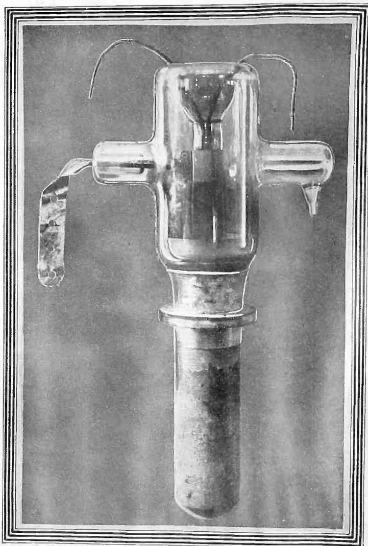
This New Tube Transmits 15 kw. on 6 Meters. Such Power Never Before Was Radiated on Short Waves. The Tube Cooks Food by Radiation. See Page 17.
