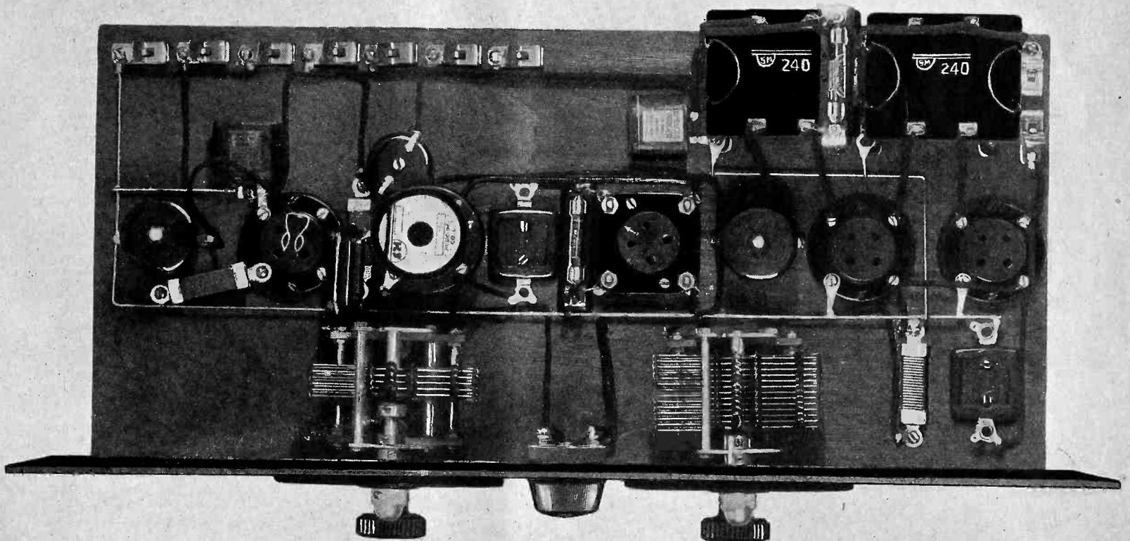
A screen grid RF tube is used ahead of the detector in this brand-new model short-wave set. See page 3.
