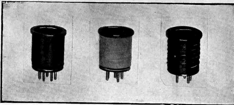
THREE OF THE SHORT WAVE COILS IN THE S-M SET OF COILS. LEFT IS THE 131-V, MIDDLE 131-W AND RIGHT 131-T.
