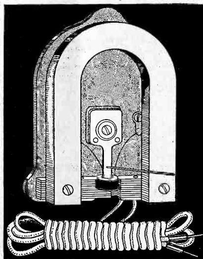
This unit has a full floating armature, which means that armature is mounted so that it acts like a plunger between two sets of magnets or pole pieces. As the magnetization of the armature changes under the influence of the signal it plunges first toward one pair of pole pieces and then toward the other.
