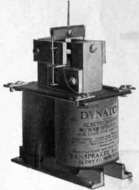
THE RUGGED AND POWERFUL ELECTRO-MAGNETIC UNIT USED IN BUILDING THE ELECTRO-DYNAMIC SPEAKER.
