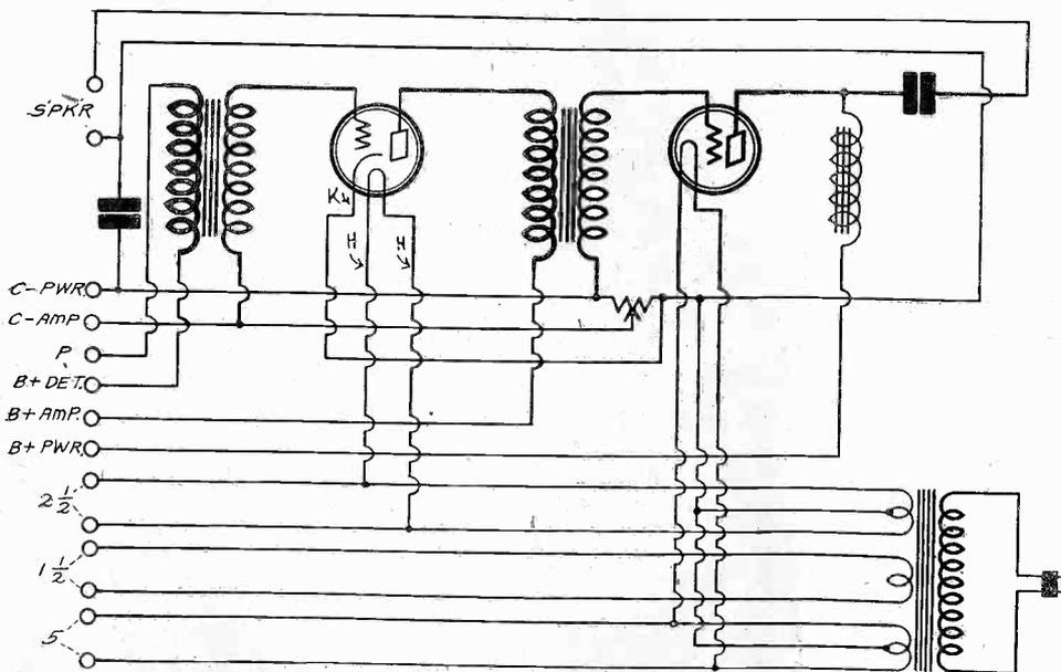
A SCIENTIFIC CIRCUIT DESIGN FOR A TWO-STAGE AC AUDIO AMPLIFIER, WITH FILAMENT TRANSFORMER AND FILTERED OUTPUT AND BUILT-IN C SUPPLY. THE B VOLTAGES ARE TO BE RECEIVED BY THIS UNIT AND THE FILAMENT VOLTAGES ARE TO BE DELIVERED BY IT TO THE TUNER. THE TUBES USED ARE ONE —26 AND ONE 112 OR —71. NOTE THAT THE MIDTAP OF THE  $2\frac{1}{2}$ -VOLT WINDING IS MADE POSITIVE IN RESPECT TO THE CATHODE. THIS GREATLY REDUCES HUM.
