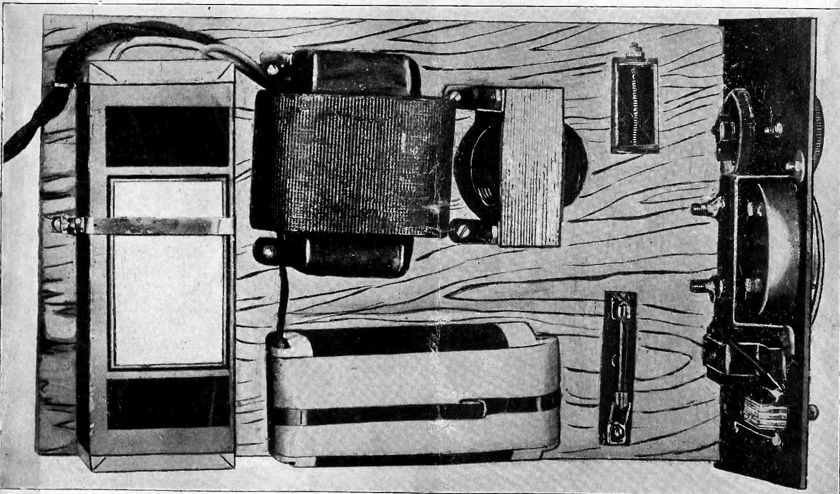
It is very easy to make a DC eliminator for supplying "A" and "B" voltages and currents. View of one is shown above. See page 3.
