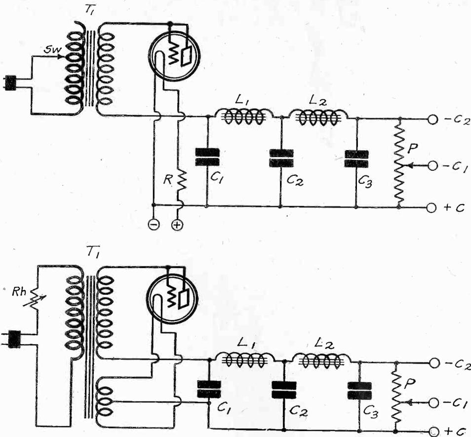
THE CIRCUIT DIAGRAM OF A SIMPLE C BATTERY ELIMINATOR UTILIZING A —99 TYPE TUBE FOR RECTIFICATION. (FIG. 1, TOP) THE FILAMENT OF RECTIFIER IS HEATED FROM RECEIVER STORAGE BATTERY. THE CIRCUIT USING AN AC HEATED TUBE FOR RECTIFICATION. (FIG. 2, LOWER) THE VOLTAGE IS REGULATED WITH A RHEOSTAT RH IN THE PRIMARY OF THE SUPPLY TRANSFORMER.
