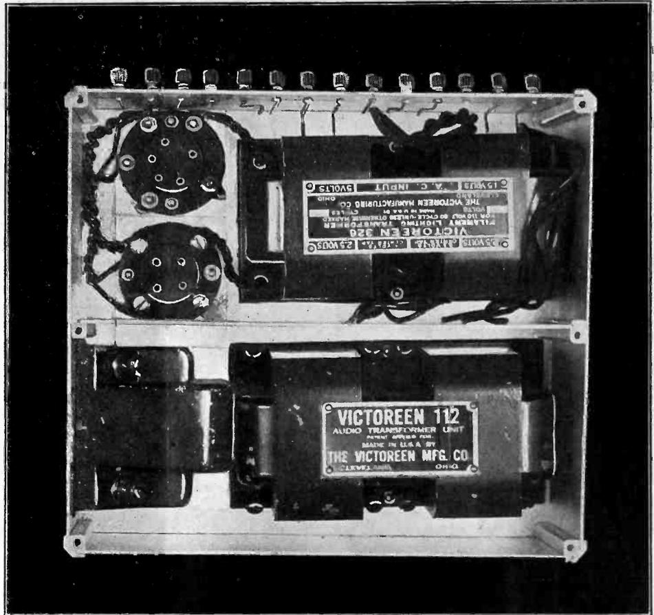
EXACT PLACEMENT OF PARTS PERMITS PARTITIONING THE FILAMENT TRANSFORMER AND TWO SOCKETS FROM THE TWO-STAGE AUDIO COUPLING AND THE OUTPUT CHOKE (LOWER LEFT). NOTE THAT THE CHOKE IS "HUNG ON THE WALL."
