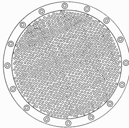
THE STATOR PLATE OF THE CONDENSER SPEAKER SHOULD BE PERFORATED, TO LET THE AIR THROUGH.
