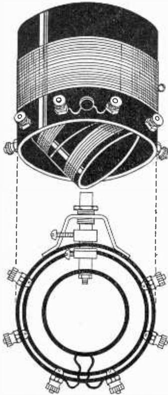
Model 5HT. High impedance 3-circuit tuner, to work out of a screen grid RF tube. For .0005 mfd. ....\$3.00
