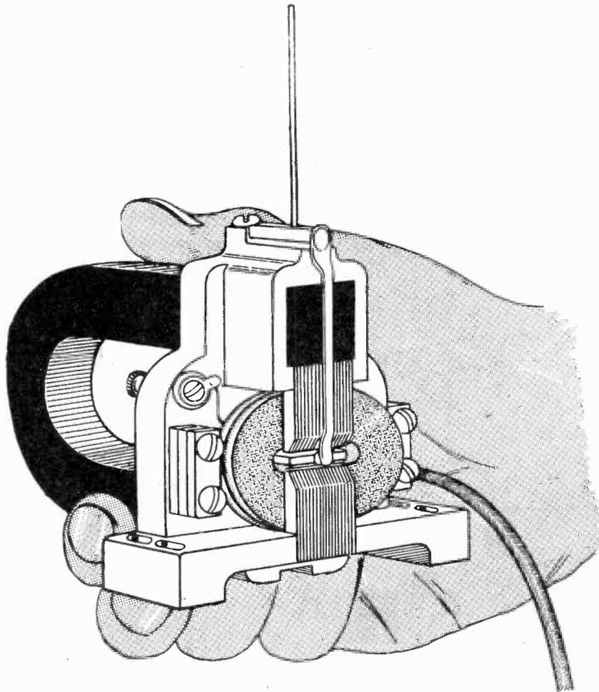
Any degree of volume is kept well in hand by the new HBH loudspeaker unit, for cones, cloth diaphragm speakers, etc. The unit is shown full size.
